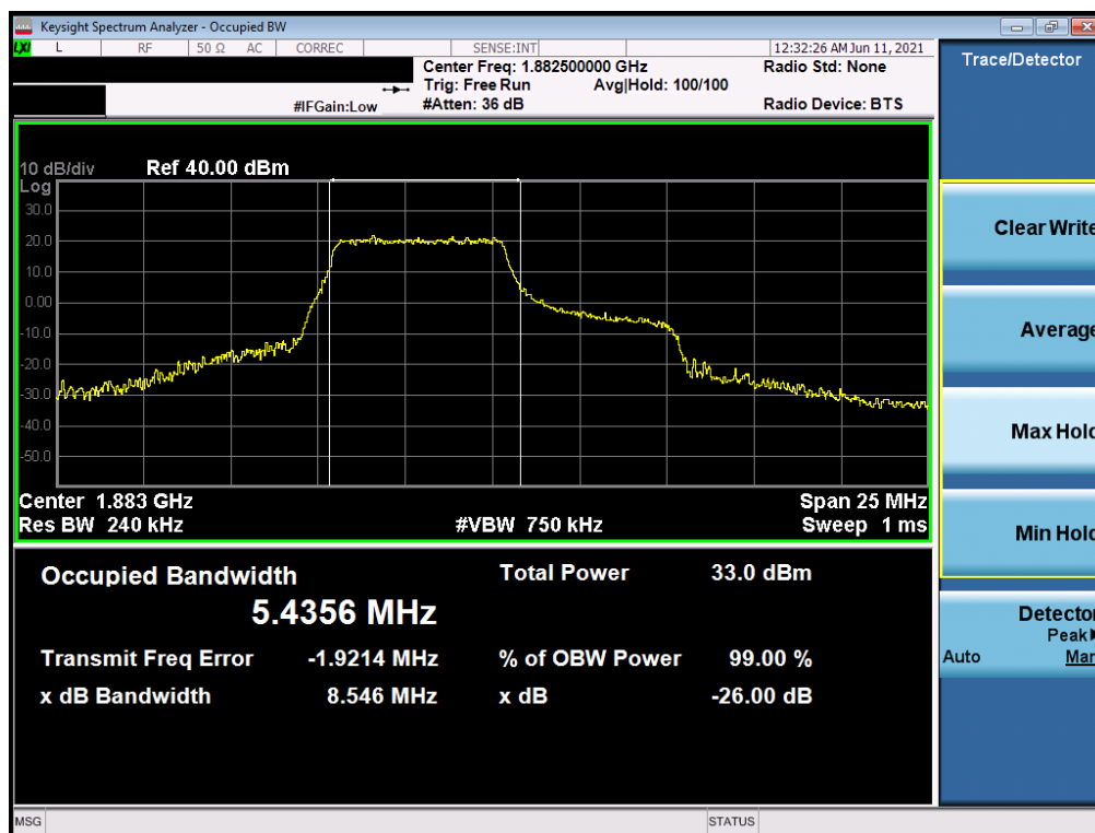
Plot 7-8. Occupied Bandwidth Plot (LTE Band 25/2 - 10MHz 16-QAM - Full RB Configuration)
