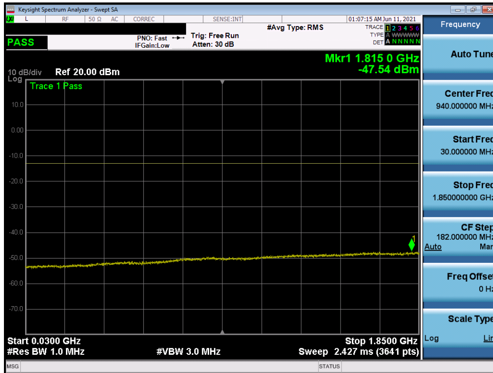
Plot 7-20. Conducted Spurious Plot (LTE Band 25/2 - 20MHz QPSK - RB Size 1, RB Offset 0 - High Channel)
