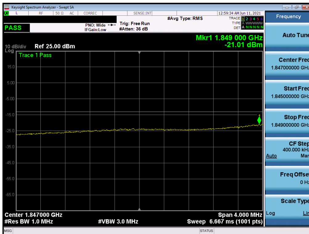
Plot 7-49. Extended Lower Band Edge Plot (LTE Band 25 – 15MHz QPSK – Full RB Configuration)
