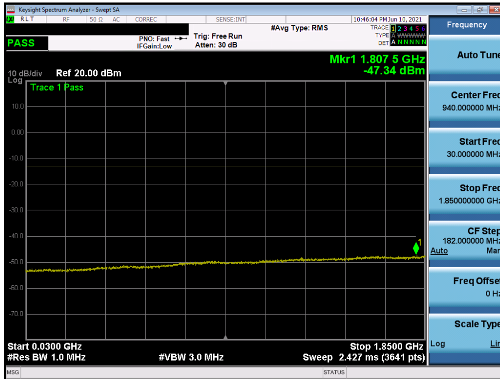
Plot 7-29. Conducted Spurious Plot (WCDMA Ch. 9538)
