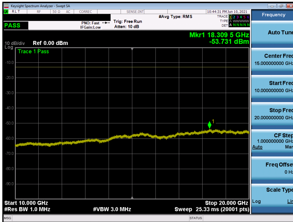
Plot 7-25. Conducted Spurious Plot (WCDMA Ch. 9262)
