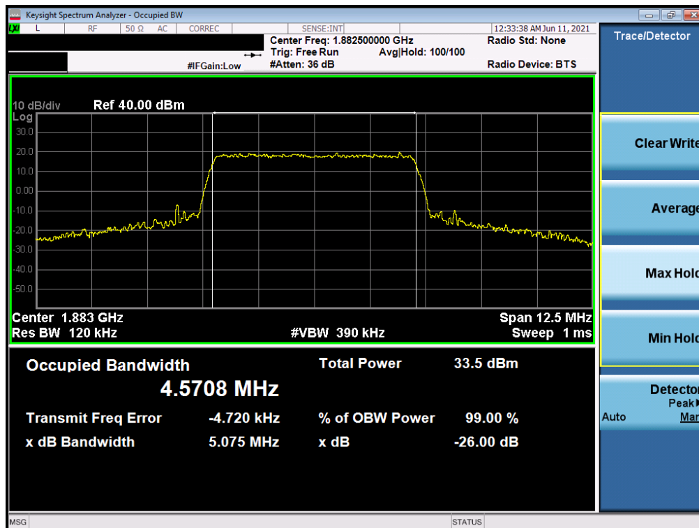
Plot 7-6. Occupied Bandwidth Plot (LTE Band 25/2 - 5MHz 16-QAM - Full RB Configuration)
