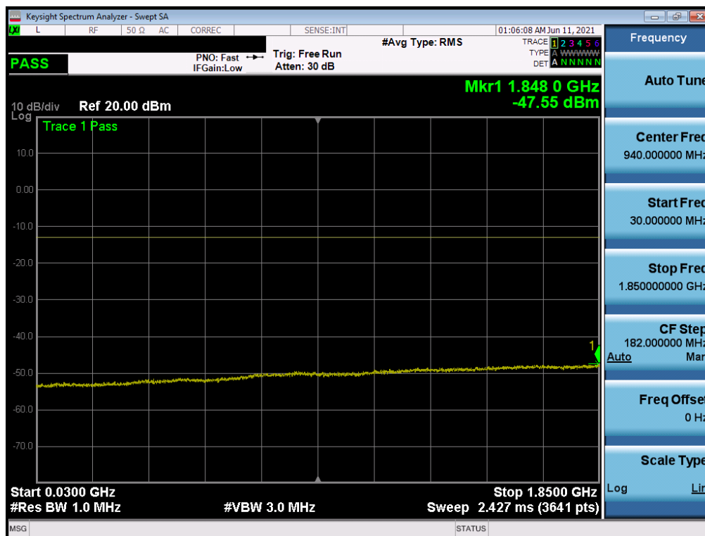
Plot 7-17. Conducted Spurious Plot (LTE Band 25/2 - 20MHz QPSK - RB Size 1, RB Offset 0 - Mid Channel)
