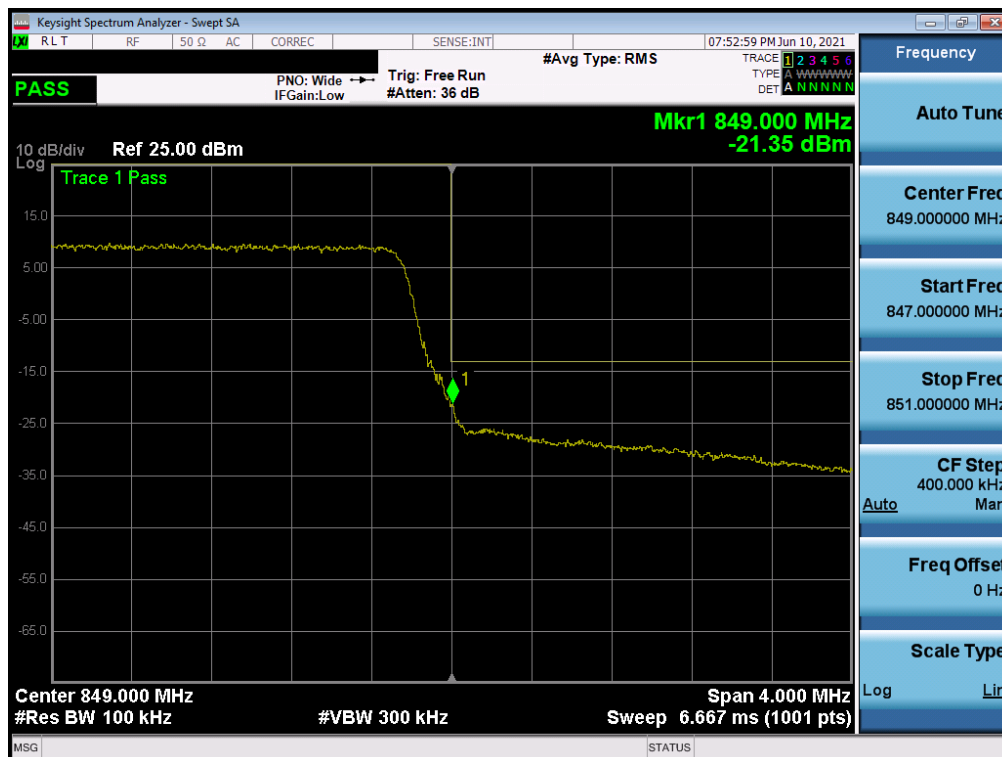
Plot 7-33. Upper BE Plot (LTE Band 5 - 5MHz QPSK – Full RB Configuration)
