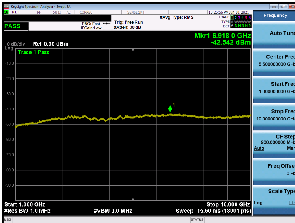
Plot 7-24. Conducted Spurious Plot (WCDMA Ch. 4183)
