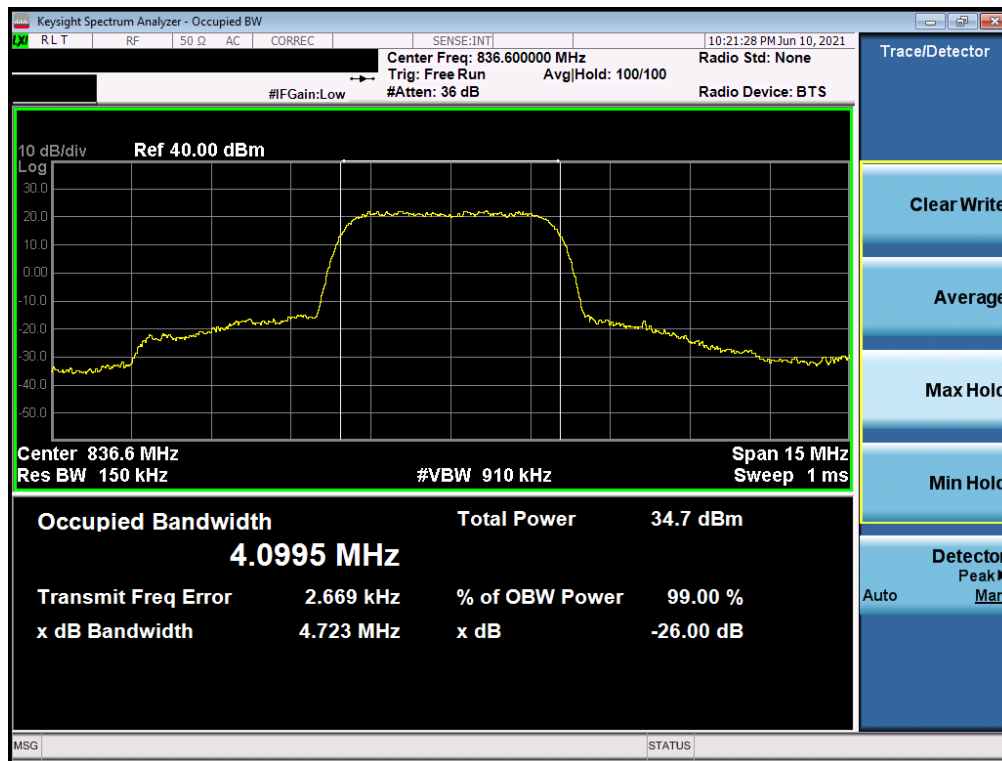
Plot 7-9. Occupied Bandwidth Plot (WCDMA, Ch. 4183)
