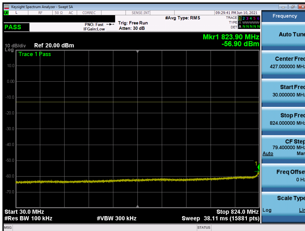
Plot 7-13. Conducted Spurious Plot (LTE Band 26/5 - 10MHz QPSK - RB Size 1, RB Offset 0 - Mid Channel)
