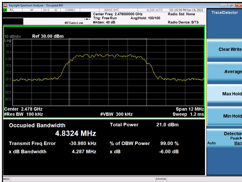
Plot 7-6. 6dB Bandwidth & 99% OBW Plot (Bluetooth (HDR8), 8Mbps, ePA – Ch. 75)
