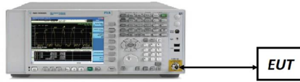
Figure 7-1. Test Instrument & Measurement Setup
