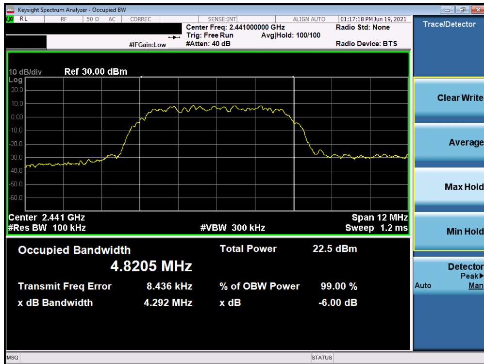
Plot 7-5. 6dB Bandwidth & 99% OBW Plot (Bluetooth (HDR8), 8Mbps, ePA – Ch. 38)
