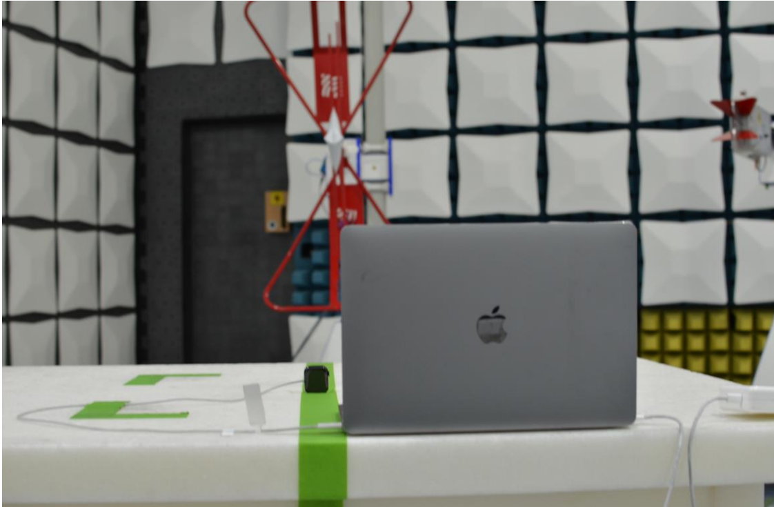
Figure 19: 30MHz-960MHz Test Setup (Rear View)
