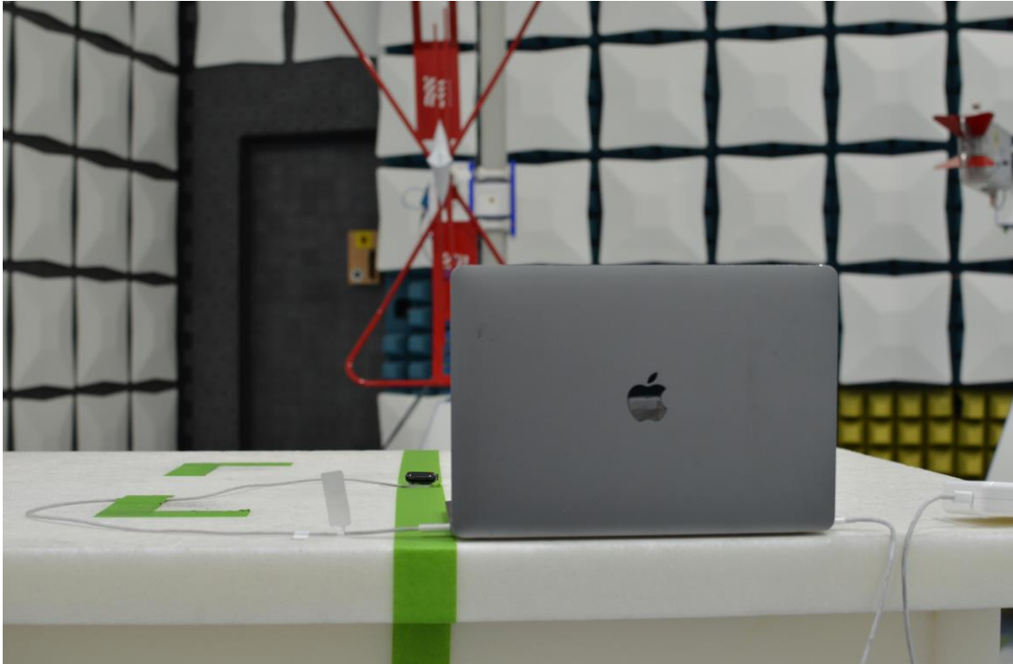
Figure 15: 30MHz-1GHz Test Setup (Rear View)
