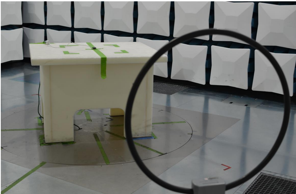
Figure 20: 9kHz-30MHz Test Setup (Front View)
