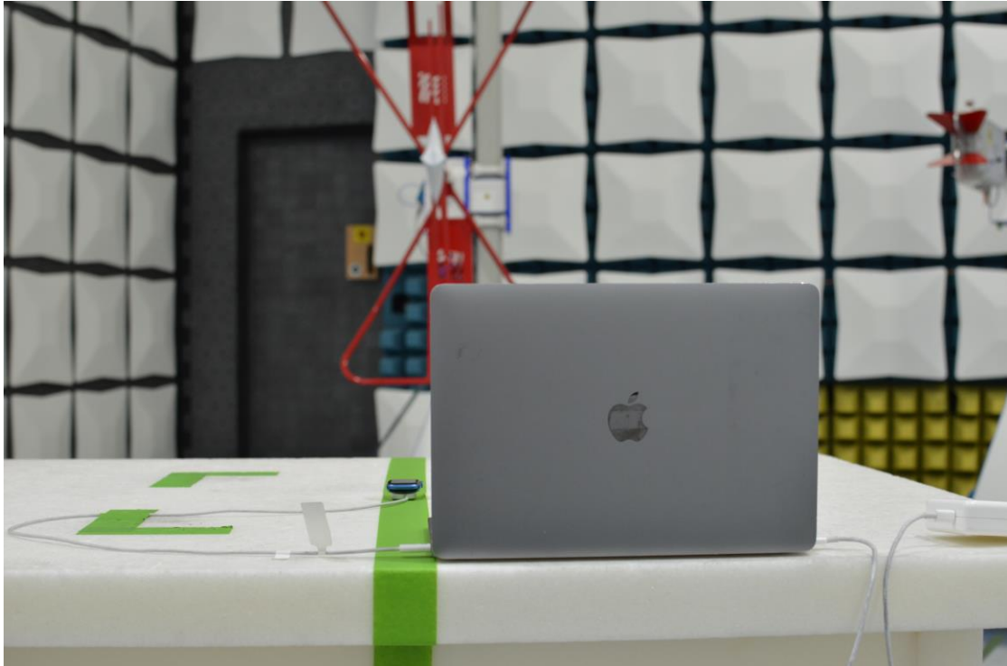
Figure 15: 30MHz-960MHz Test Setup (Rear View)
