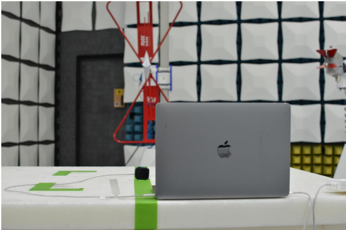
Figure 17: 30MHz-960MHz Test Setup (Rear View)
