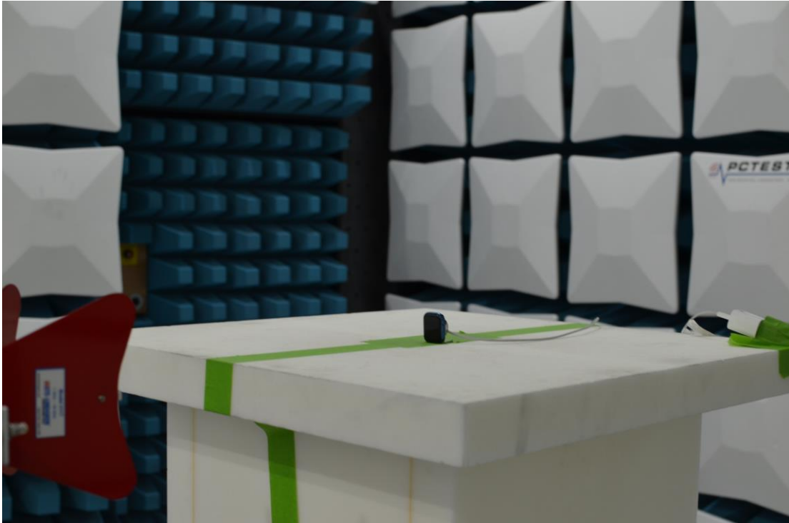
Figure 7: Above 960MHz Test Setup
