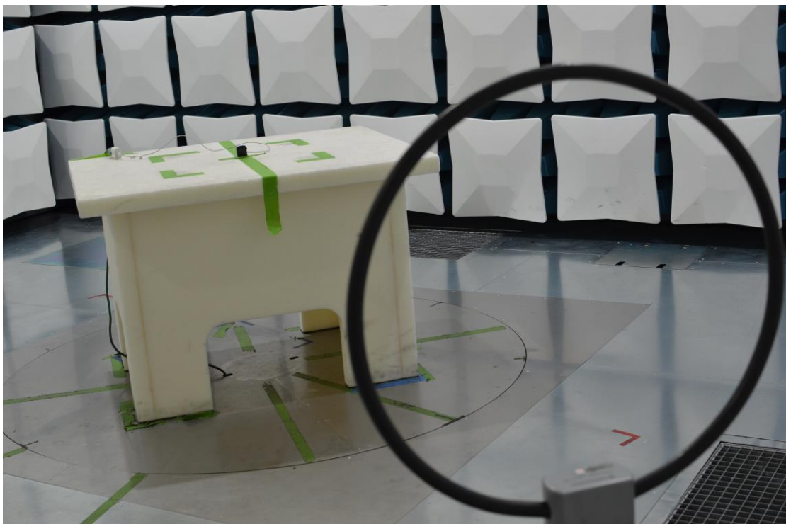
Figure 22: 9kHz-30MHz Test Setup (Front View)
