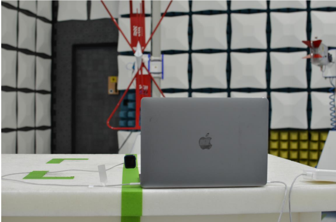
Figure 19: 30MHz-960MHz Test Setup (Rear View)
