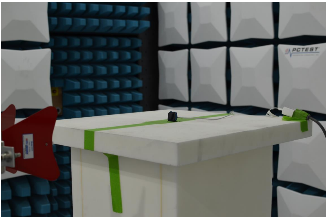
Figure 6: Above 960MHz Test Setup
