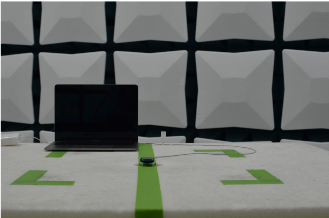
Figure 14: 30MHz-960MHz Test Setup (Front View)
