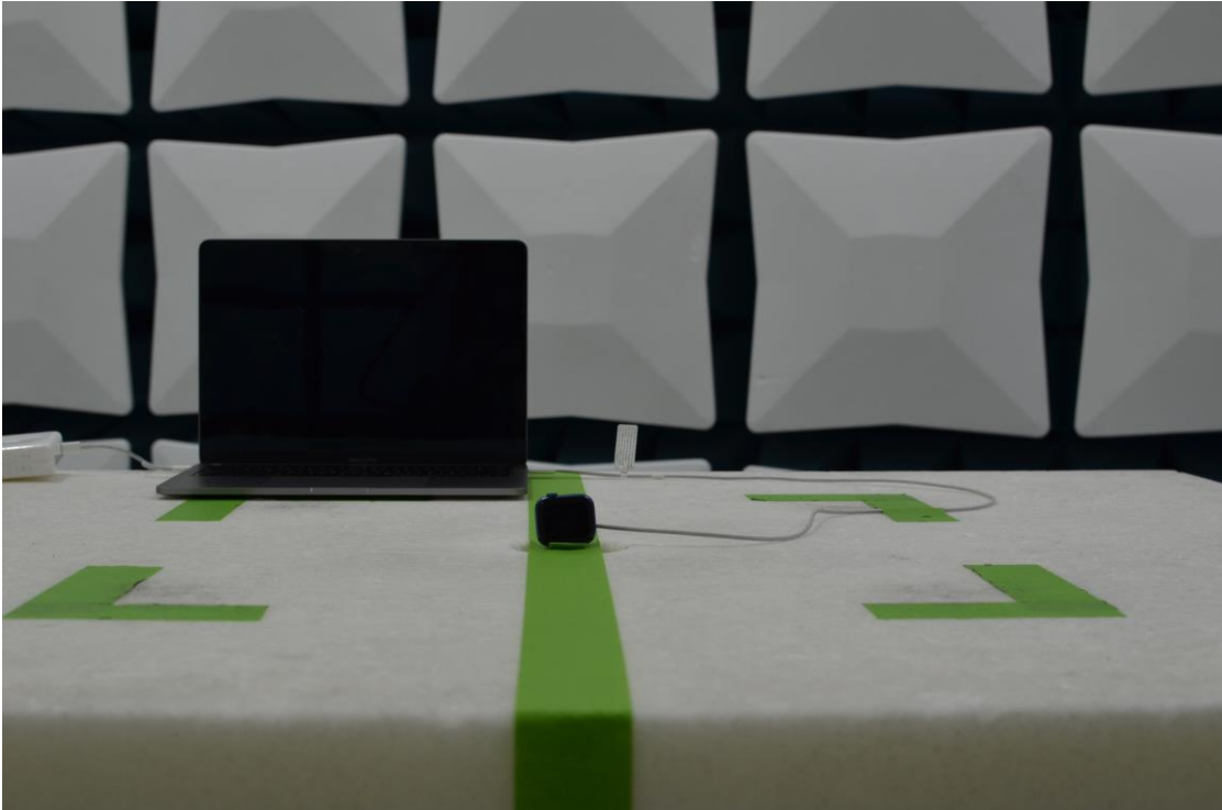
Figure 19: 30MHz-1GHz Test Setup (Front View)
