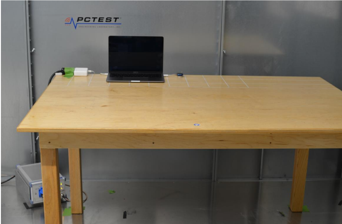
Figure 3: AC Line Conducted Emissions (Front View)
