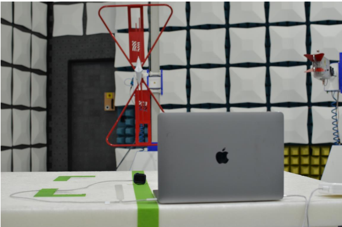
Figure 20: 30MHz-1GHz Test Setup (Rear View)
