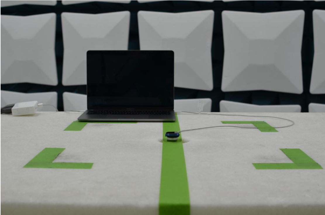
Figure 17: 30MHz-1GHz Test Setup (Front View)
