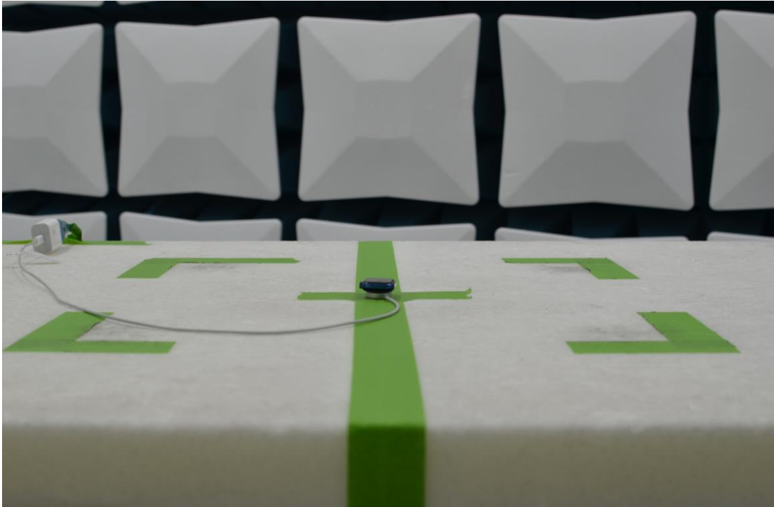
Figure 11: 30MHz-1GHz Test Setup (Front View)
