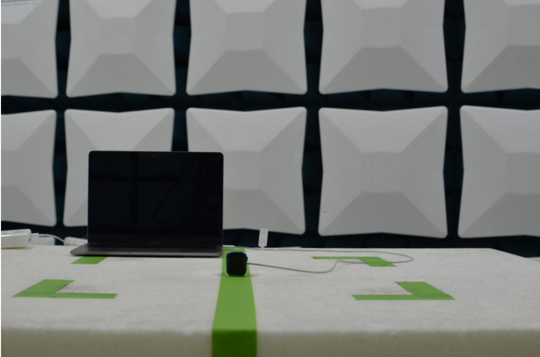
Figure 21: 30MHz-1GHz Test Setup (Front View)
