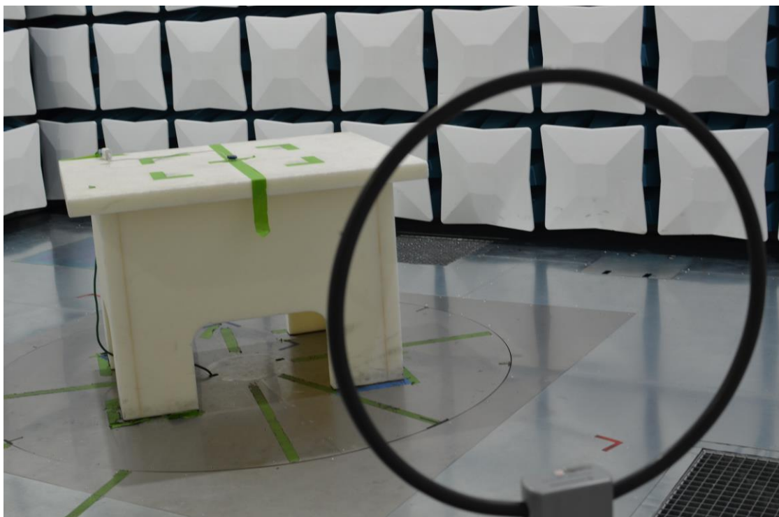
Figure 23: 9kHz-30MHz Test Setup (Front View)
