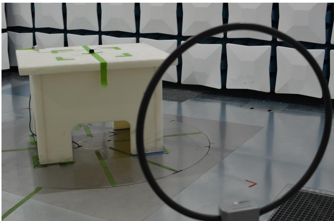
Figure 24: 9kHz-30MHz Test Setup (Front View)
