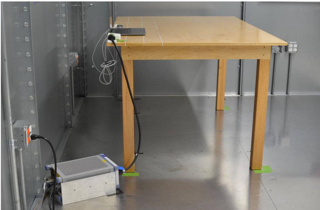
Figure 4: AC Line Conducted Emissions (Side View)
