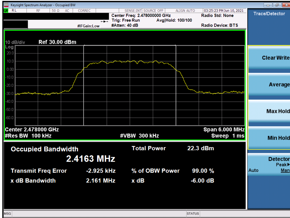
Plot 7-3. 6dB and 99% OBW Plot (Bluetooth (HDR4), 4Mbps, ePA – Ch. 75)
