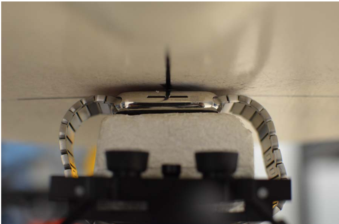
SAR Test Setup Photo 14: Stainless Steel with Metal Links Wristband, Back Side at 0.0 cm
