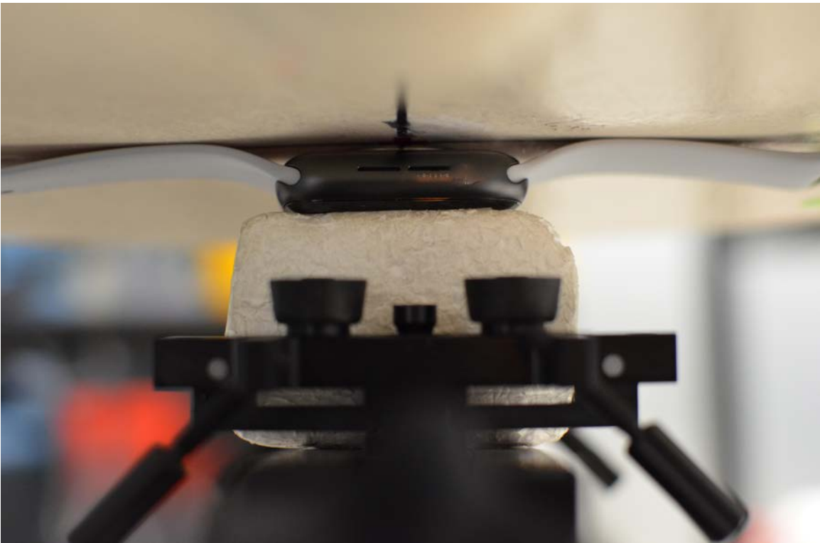
SAR Test Setup Photo 10: Aluminum with Sport Wristband, Back Side at 0.0 cm
