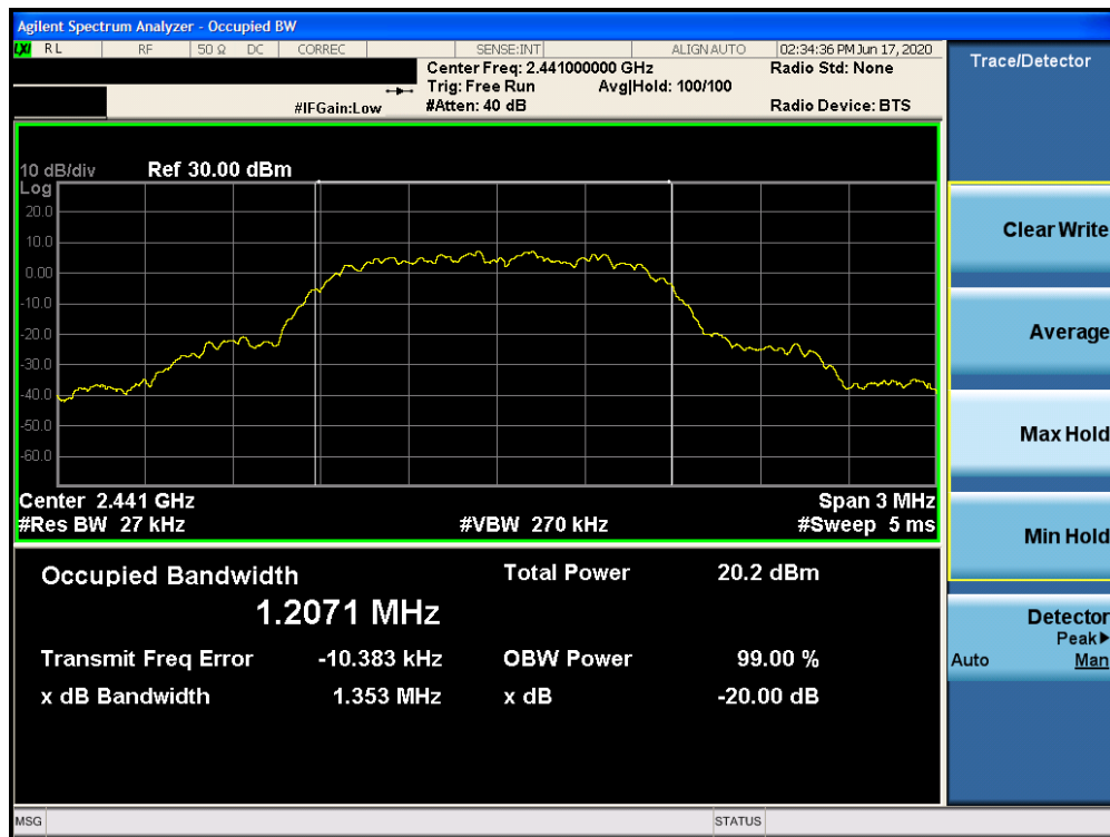
Plot 7-5. 20dB Bandwidth Plot (Bluetooth, 8DPSK, ePA – Ch. 39)
