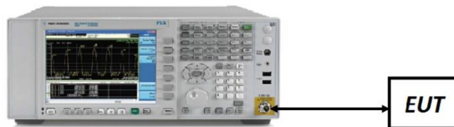
Figure 7-5. Test Instrument & Measurement Setup
