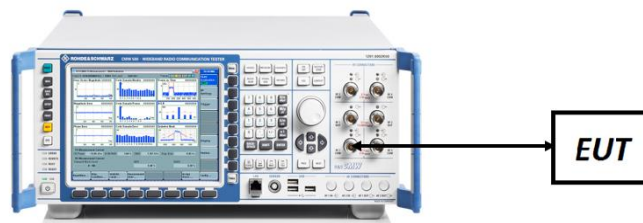
Figure 7-4. Conducted Power Measurement Setup
