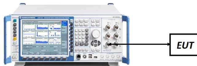
Figure 7-5. ERP/EIRP Measurement Setup
