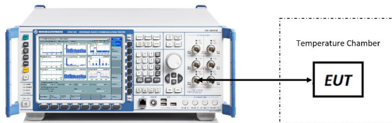
Figure 7-8. Test Instrument & Measurement Setup
