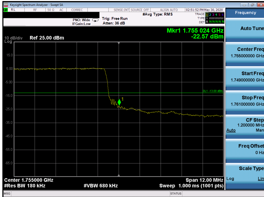
Plot 7-152. Upper Band Edge Plot (Band 4 - 15.0MHz QPSK - Full RB Configuration)
