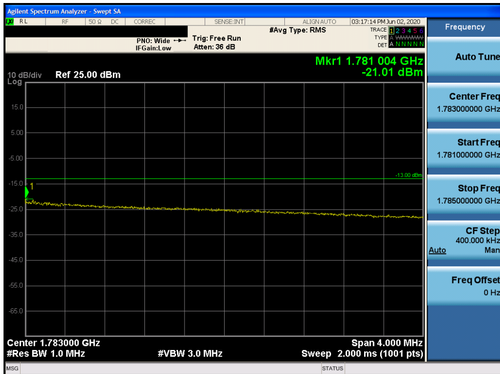
Plot 7-133. Upper Extended Band Edge Plot (Band 66 - 20.0MHz QPSK - Full RB Configuration)
