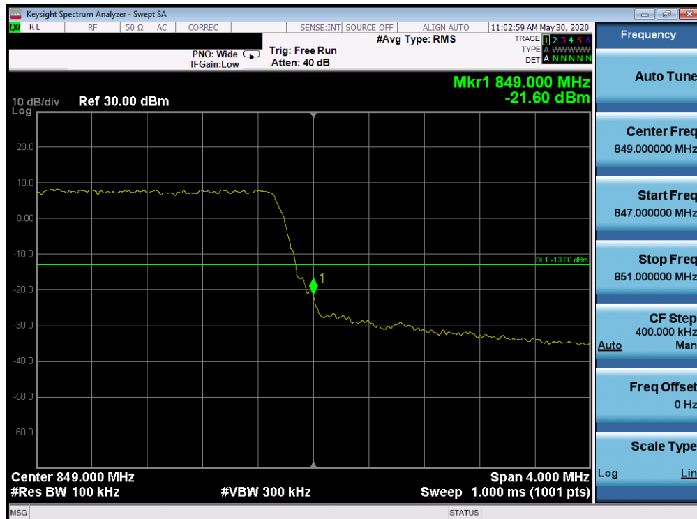
Plot 7-107. Upper Band Edge Plot (Band 5 - 5.0MHz QPSK - Full RB Configuration)
