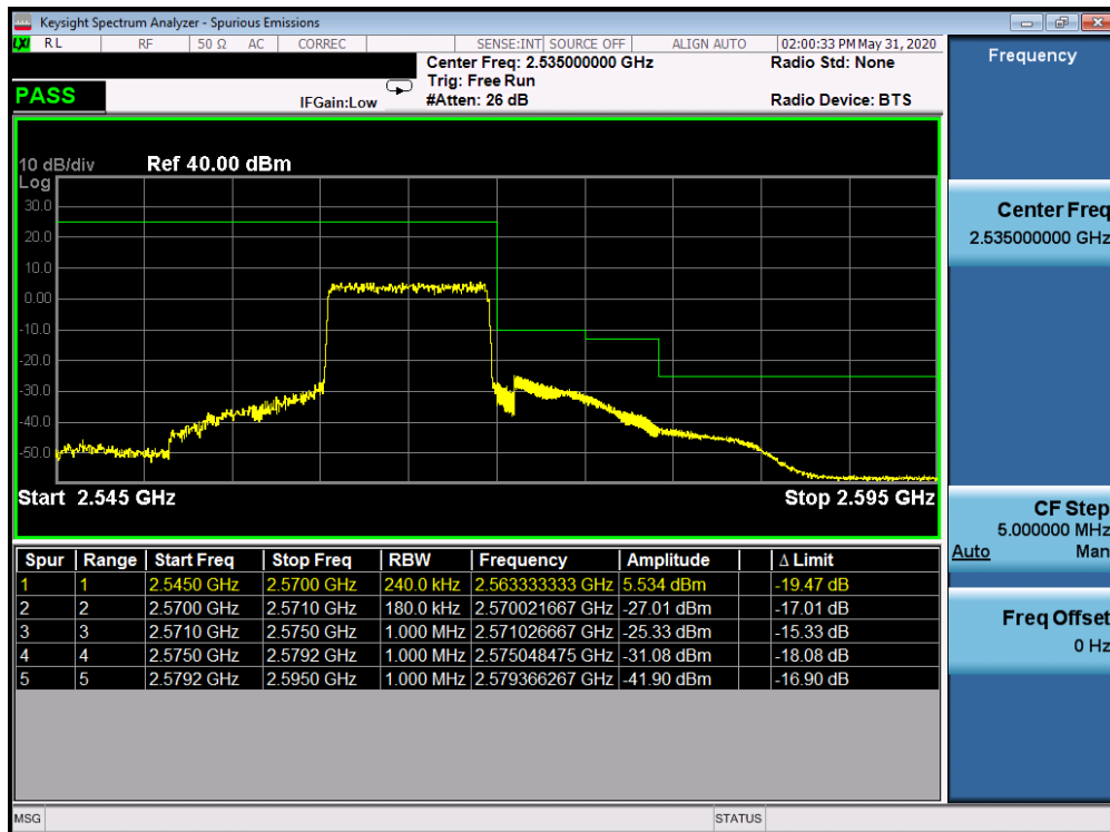
Plot 7-209. Upper ACP Plot (Band 7 - 10.0MHz QPSK - Full RB Configuration)
