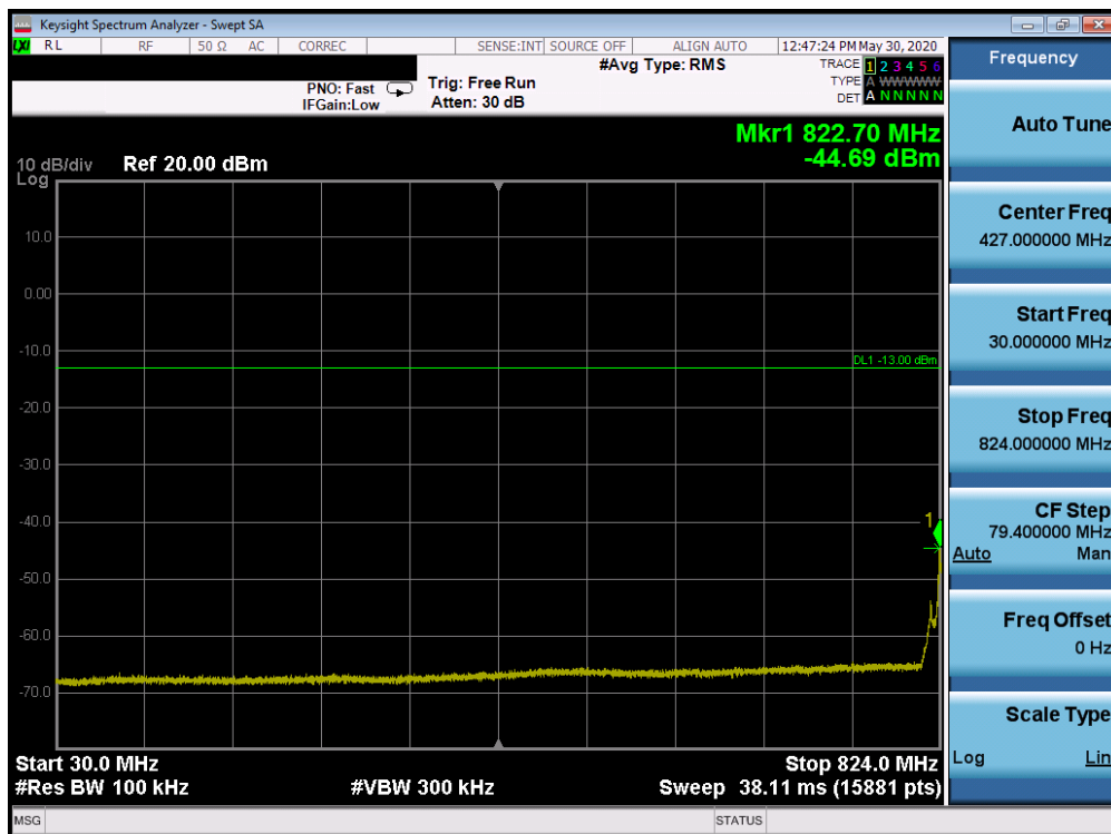
Plot 7-52. Conducted Spurious Plot (Band 26/5 - 10.0MHz QPSK - RB Size 1, RB Offset 0 - Mid Channel)
