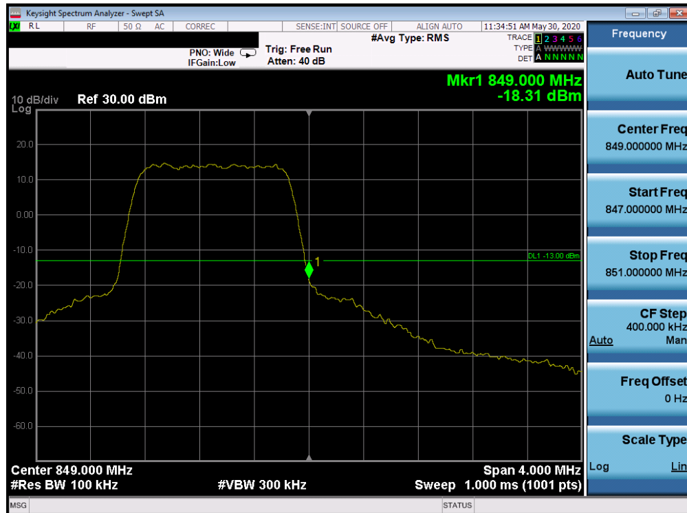
Plot 7-103. Upper Band Edge Plot (Band 5 - 1.4MHz QPSK - Full RB Configuration)
