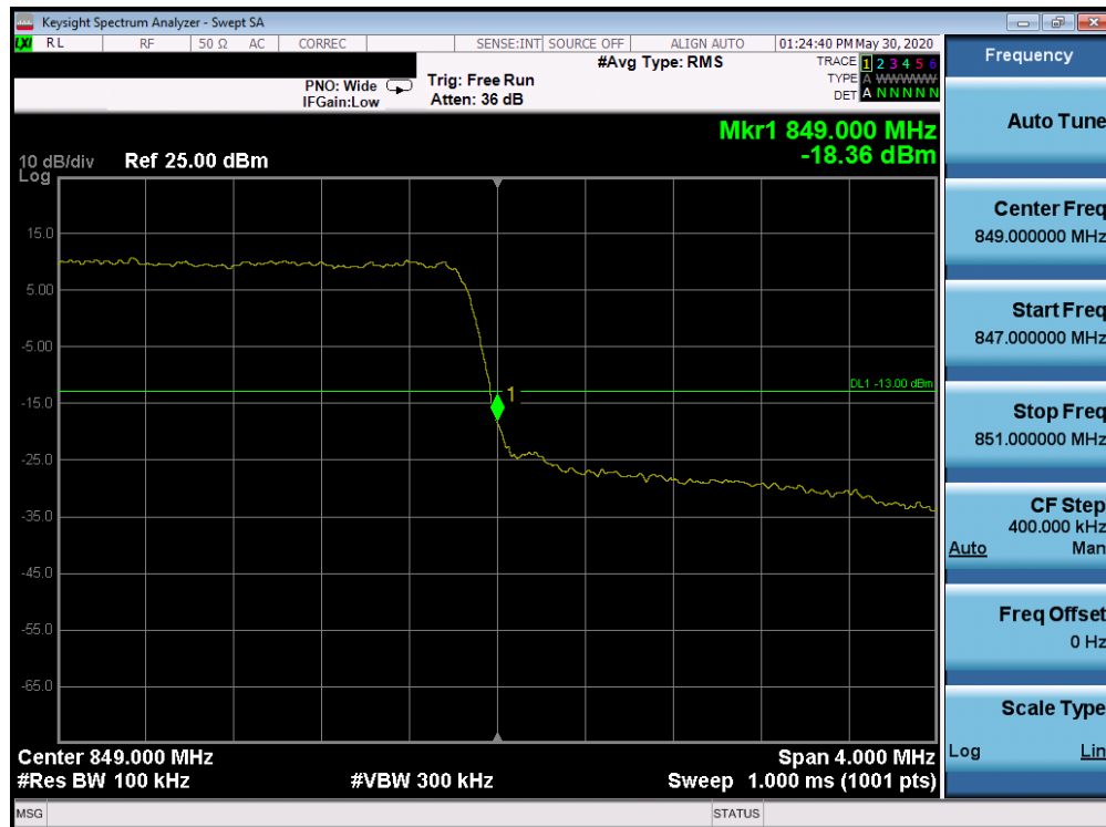
Plot 7-97. Upper Band Edge Plot (Band 26 - 3.0MHz QPSK - Full RB Configuration)
