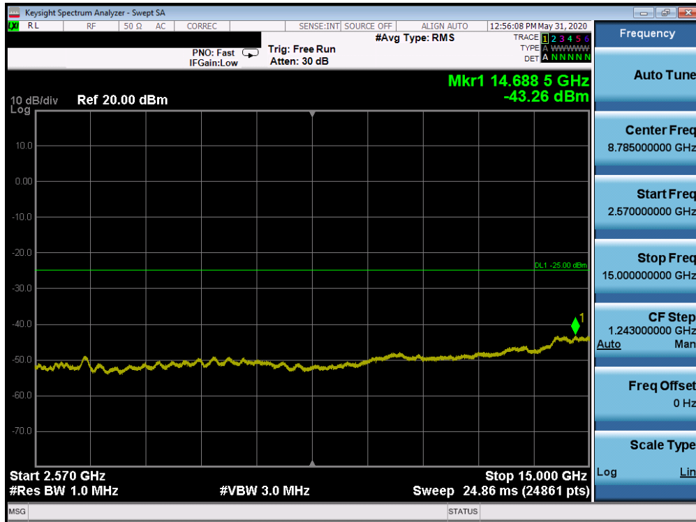
Plot 7-80. Conducted Spurious Plot (Band 7 - 20.0MHz QPSK - RB Size 1, RB Offset 0 - Mid Channel)
