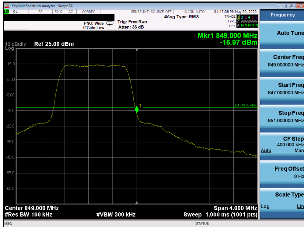
Plot 7-95. Upper Band Edge Plot (Band 26 - 1.4MHz QPSK - Full RB Configuration)
