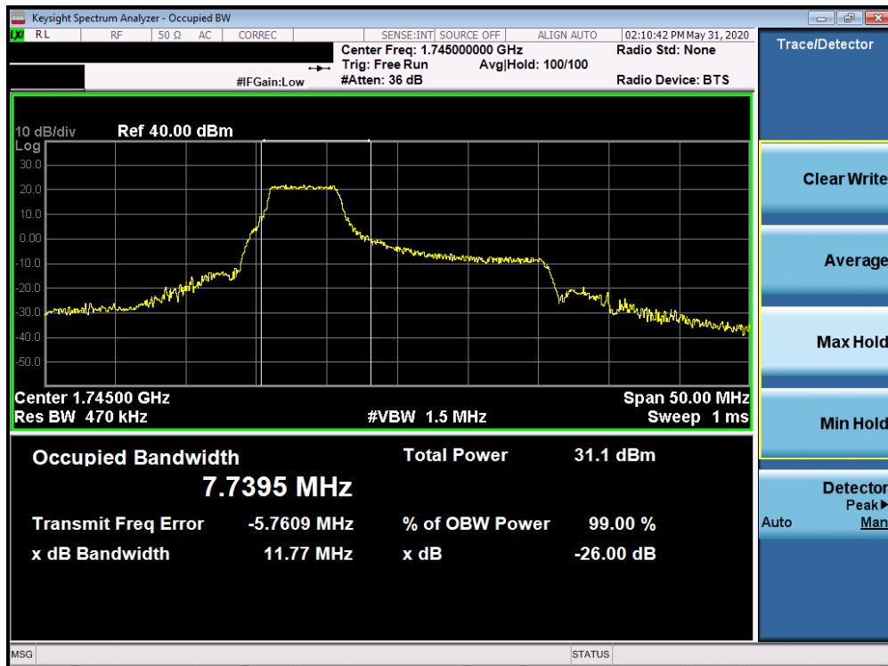
Plot 7-20. Occupied Bandwidth Plot (Band 66/4 - 20.0MHz 16-QAM - Full RB Configuration)
