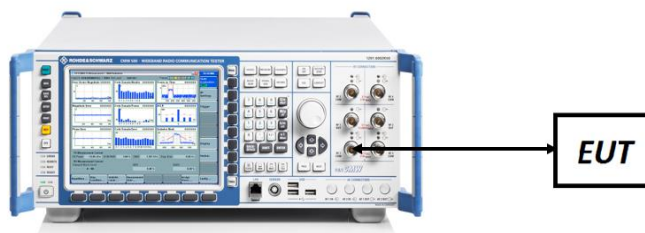
Figure 7-5. ERP/EIRP Measurement Setup
