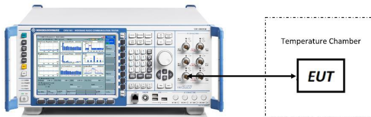
Figure 7-8. Test Instrument & Measurement Setup
