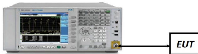
Figure 7-4. Test Instrument & Measurement Setup
