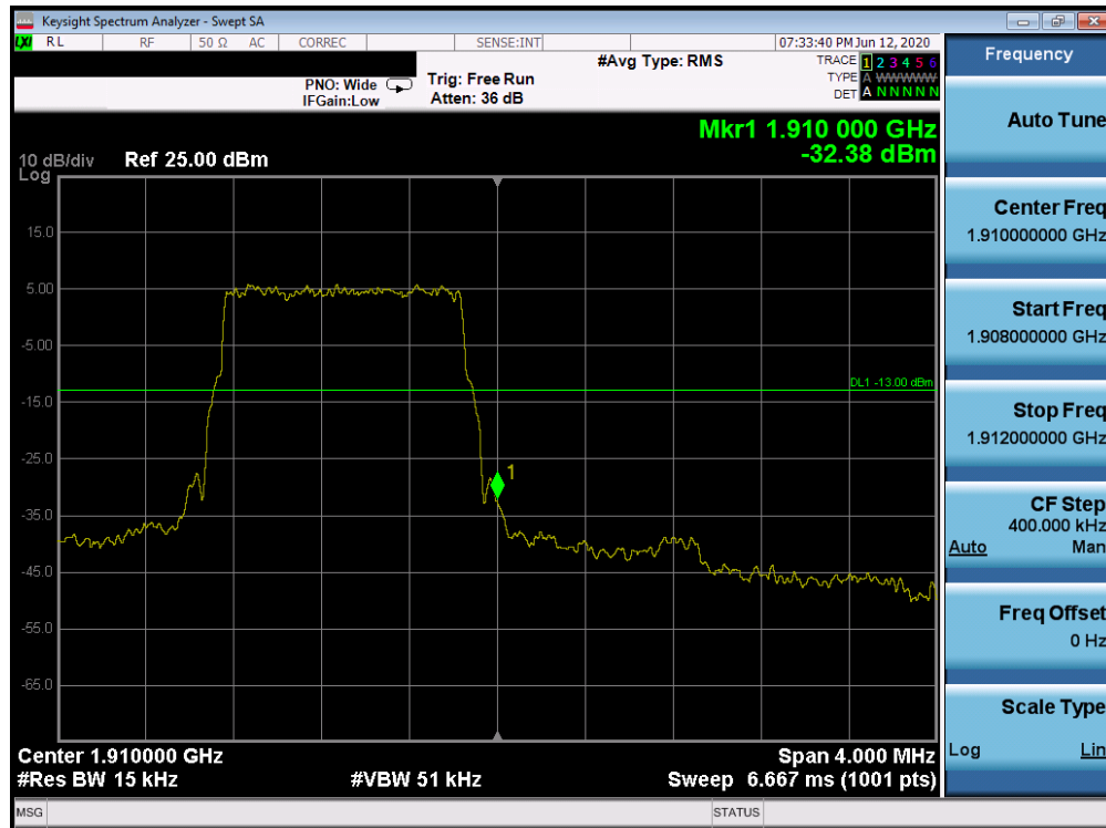
Plot 7-184. Upper Band Edge Plot (Band 2 - 1.4MHz QPSK - Full RB Configuration)
