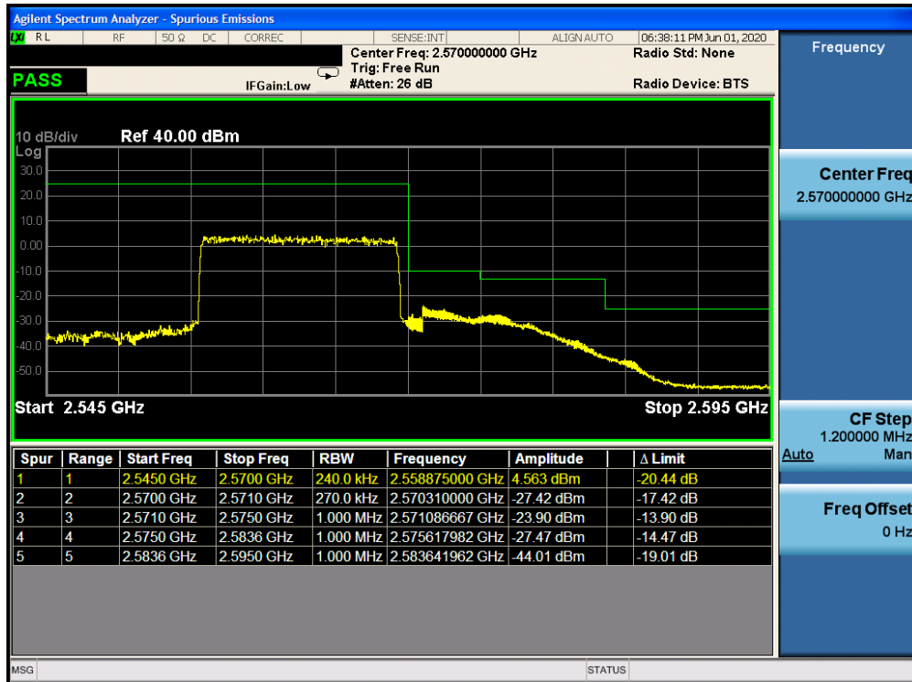
Plot 7-211. Upper ACP Plot (Band 7 - 15.0MHz QPSK - Full RB Configuration)
