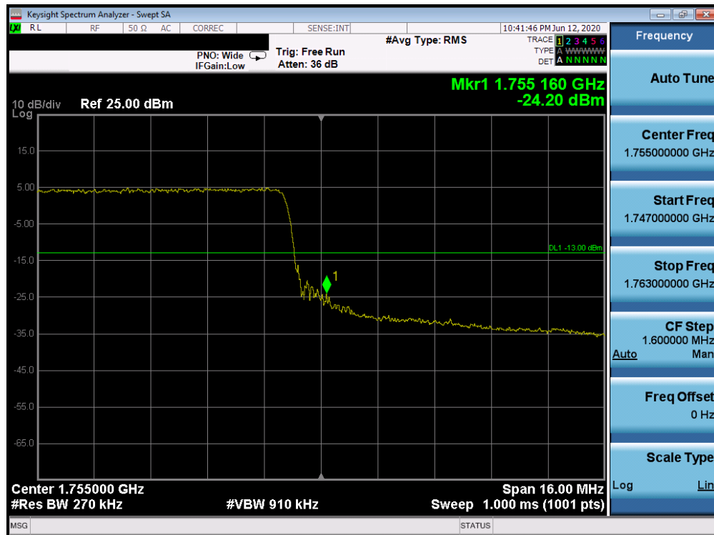
Plot 7-156. Upper Band Edge Plot (Band 4 - 20.0MHz QPSK - Full RB Configuration)
