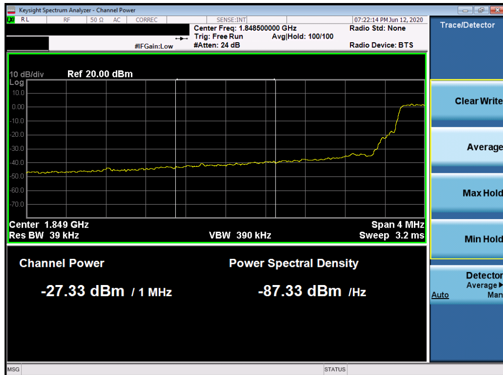
Plot 7-191. Lower Extended Band Edge Plot (Band 2 - 5.0MHz QPSK - Full RB Configuration)
