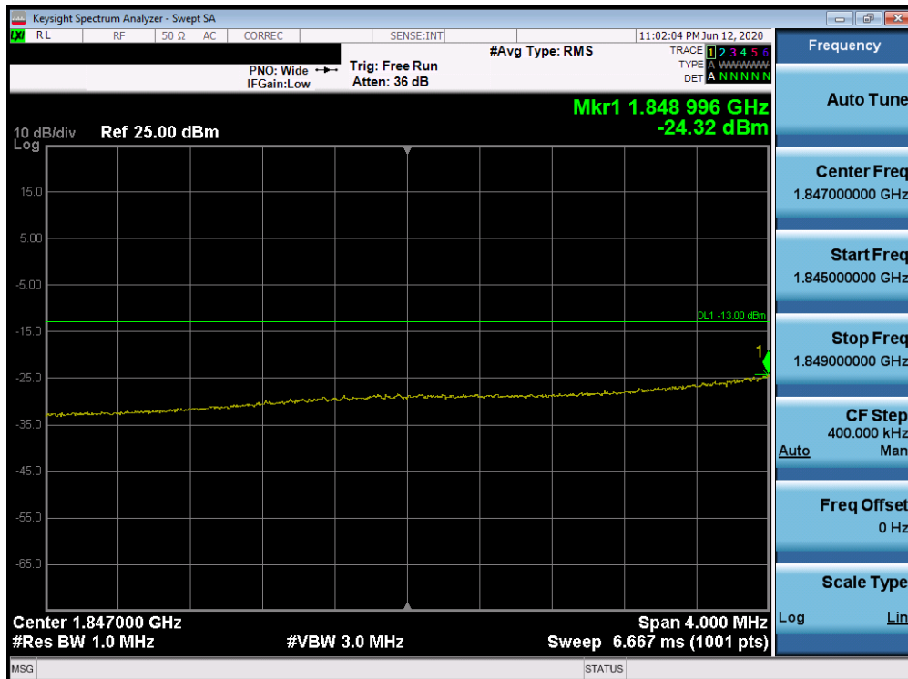
Plot 7-175. Lower Extended Band Edge Plot (Band 25 - 15.0MHz QPSK - Full RB Configuration)
