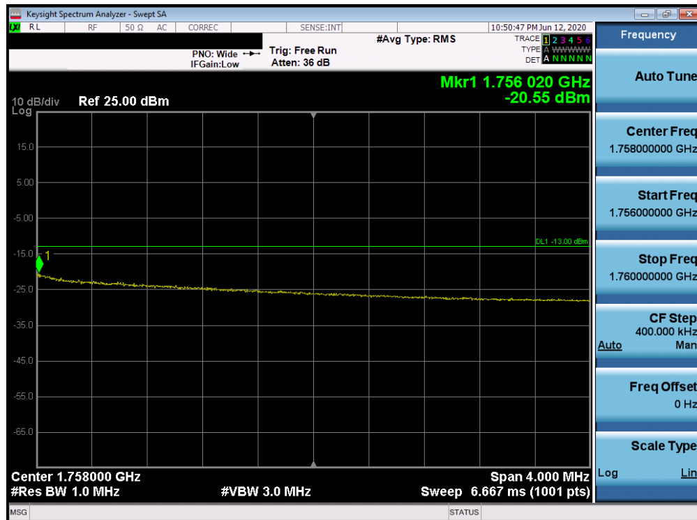
Plot 7-149. Upper Extended Band Edge Plot (Band 4 - 10.0MHz QPSK - Full RB Configuration)
