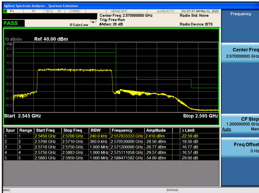
Plot 7-213. Upper ACP Plot (Band 7 - 20.0MHz QPSK - Full RB Configuration)
