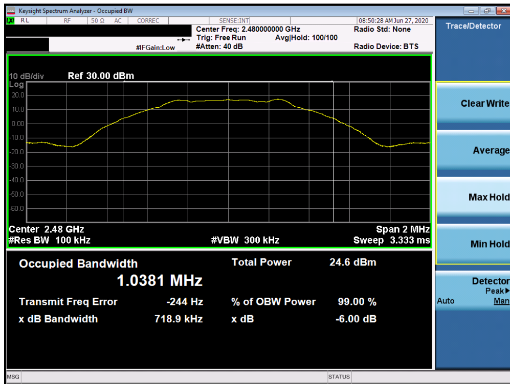
Plot 7-3. 6dB Bandwidth Plot (Bluetooth (LE), 1Mbps, ePA – Ch. 39)
