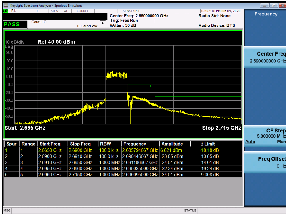
Plot 7-265. Upper ACP Plot (Band 41 - 5.0MHz QPSK - Full RB Configuration)
