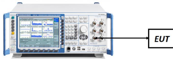
Figure 7-5. ERP/EIRP Measurement Setup
