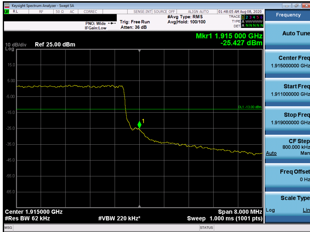
Plot 7-222. Upper Band Edge Plot (Band 25 - 10.0MHz QPSK - Full RB Configuration)
