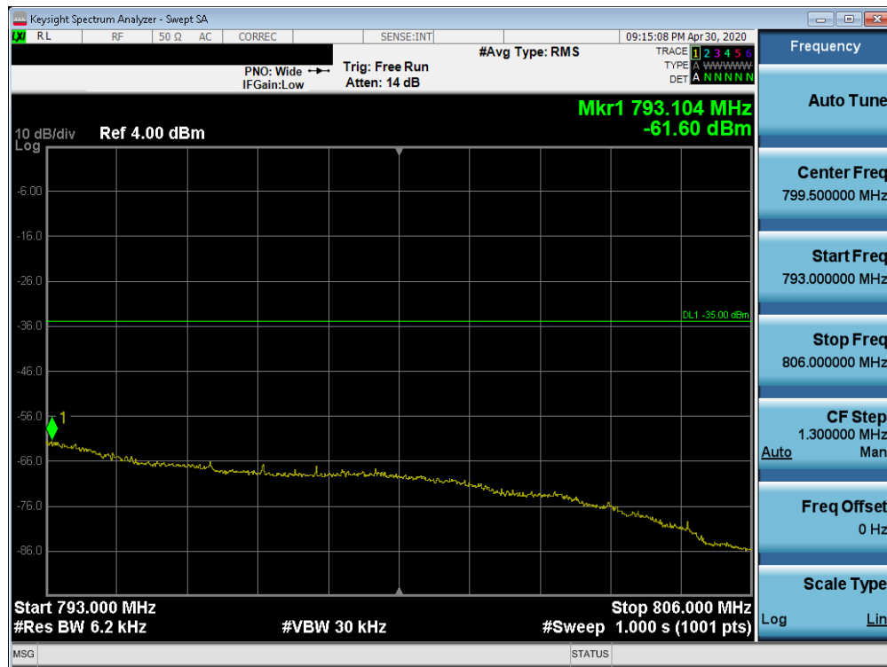
Plot 7-139. Higher Emission Mask Edge Plot (Band 13 - 5.0MHz QPSK - Full RB Configuration)
