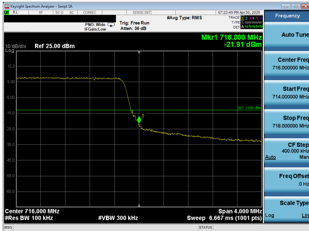
Plot 7-129. Upper Band Edge Plot (Band 12 - 5.0MHz QPSK - Full RB Configuration)
