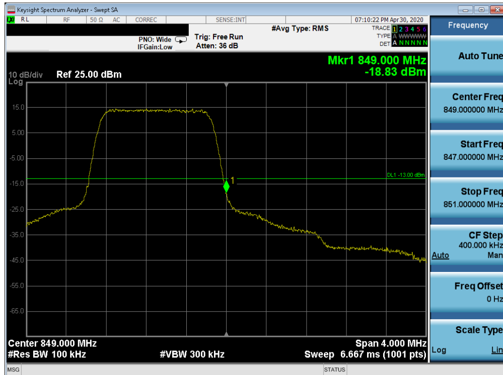
Plot 7-153. Upper Band Edge Plot (Band 5 - 1.4MHz QPSK - Full RB Configuration)
