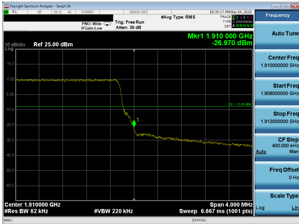
Plot 7-242. Upper Band Edge Plot (Band 2 - 5.0MHz QPSK - Full RB Configuration)
