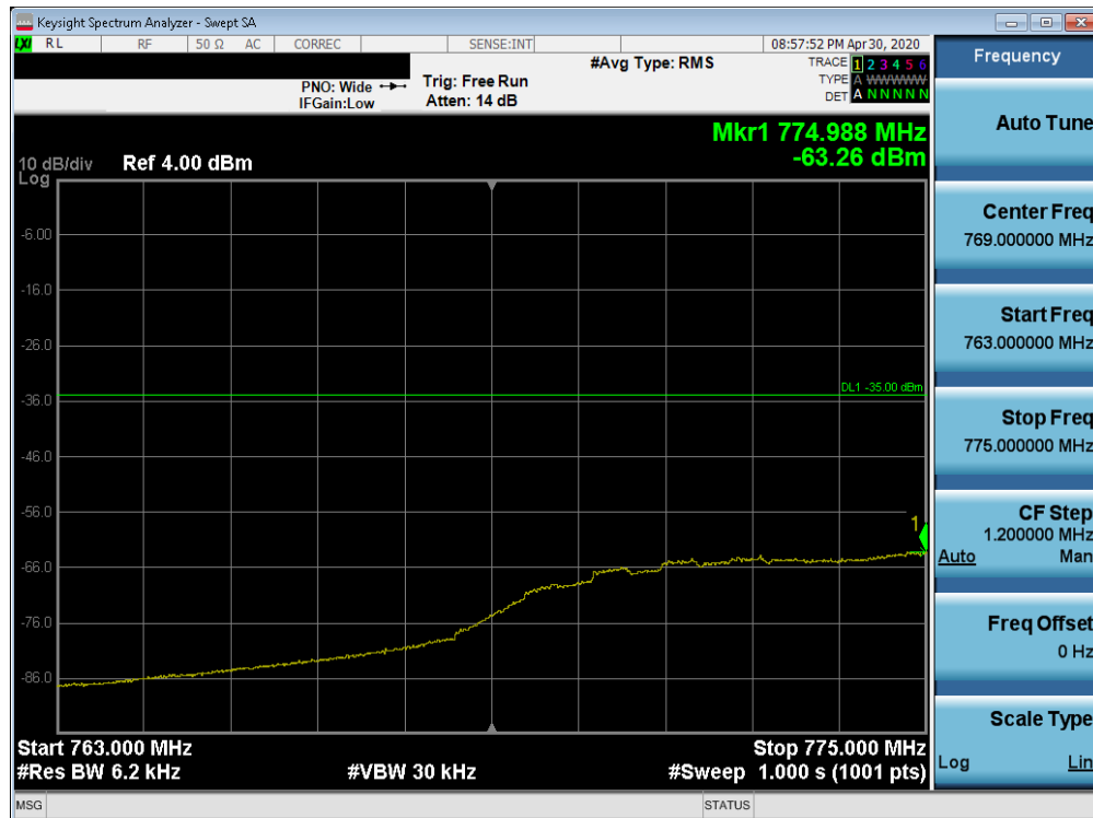
Plot 7-141. Lower Emission Mask Edge Plot (Band 13 - 10.0MHz QPSK - Full RB Configuration)
