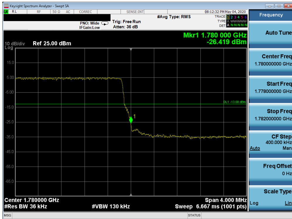
Plot 7-166. Upper Band Edge Plot (Band 66 - 3.0MHz QPSK - Full RB Configuration)
