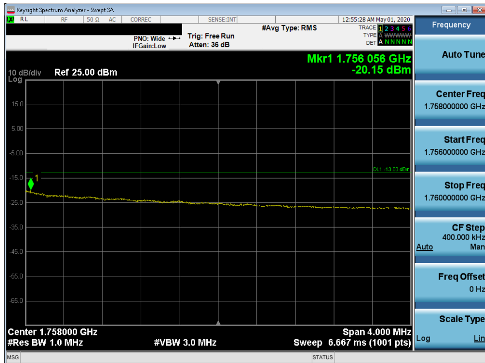
Plot 7-199. Upper Extended Band Edge Plot (Band 4 - 10.0MHz QPSK - Full RB Configuration)
