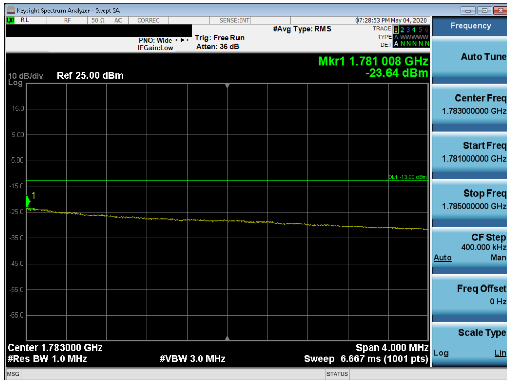
Plot 7-179. Upper Extended Band Edge Plot (Band 66 - 15.0MHz QPSK - Full RB Configuration)
