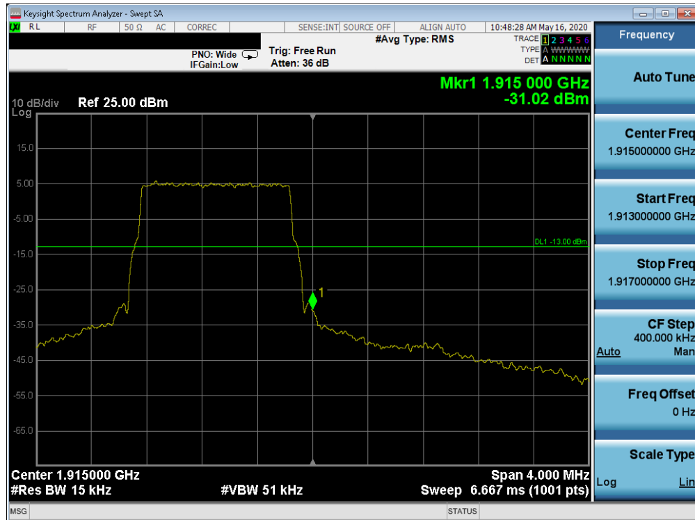
Plot 7-210. Upper Band Edge Plot (Band 25 - 1.4MHz QPSK - Full RB Configuration)
