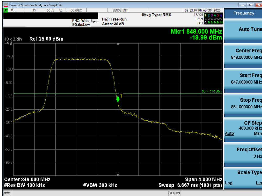
Plot 7-145. Upper Band Edge Plot (Band 26 - 1.4MHz QPSK - Full RB Configuration)
