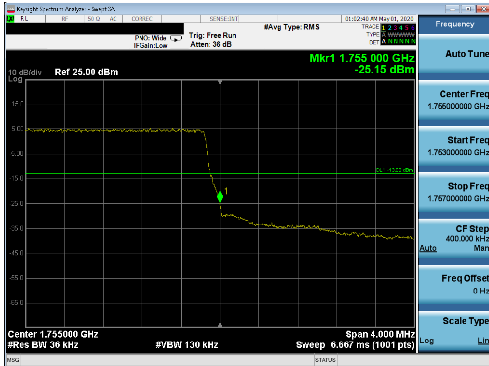
Plot 7-190. Upper Band Edge Plot (Band 4 - 3.0MHz QPSK - Full RB Configuration)
