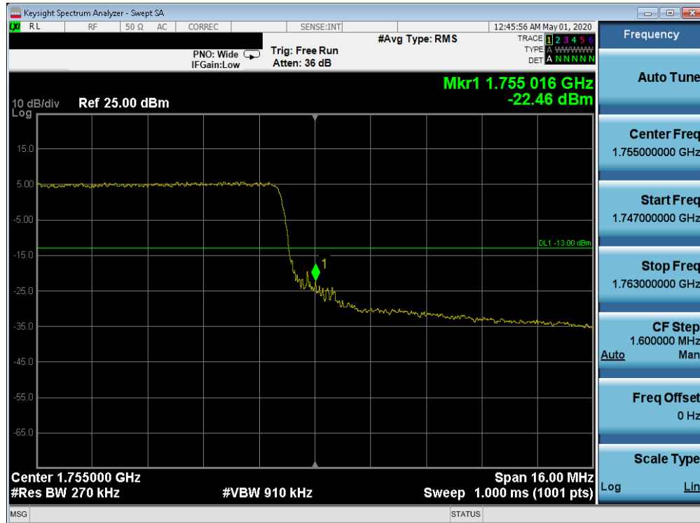
Plot 7-206. Upper Band Edge Plot (Band 4 - 20.0MHz QPSK - Full RB Configuration)
