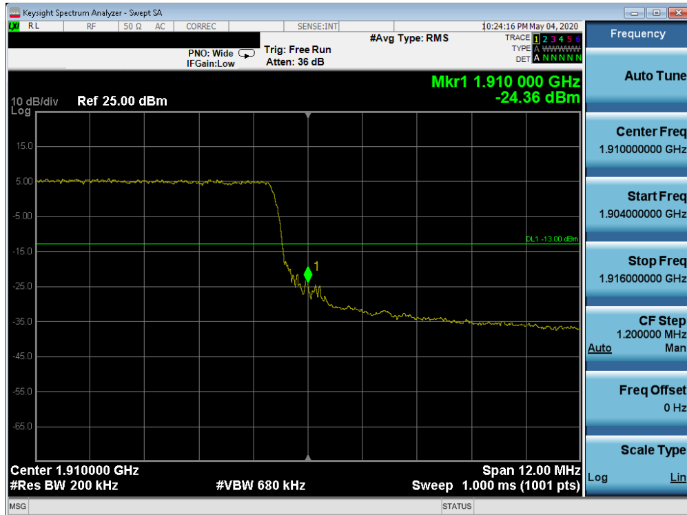
Plot 7-250. Upper Band Edge Plot (Band 2 - 15.0MHz QPSK - Full RB Configuration)
