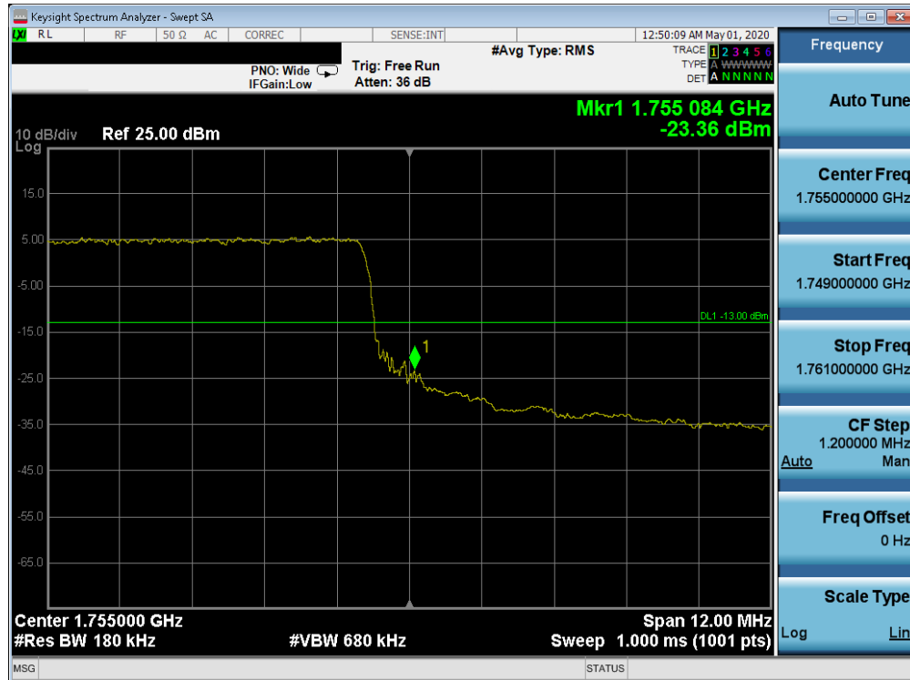
Plot 7-202. Upper Band Edge Plot (Band 4 - 15.0MHz QPSK - Full RB Configuration)
