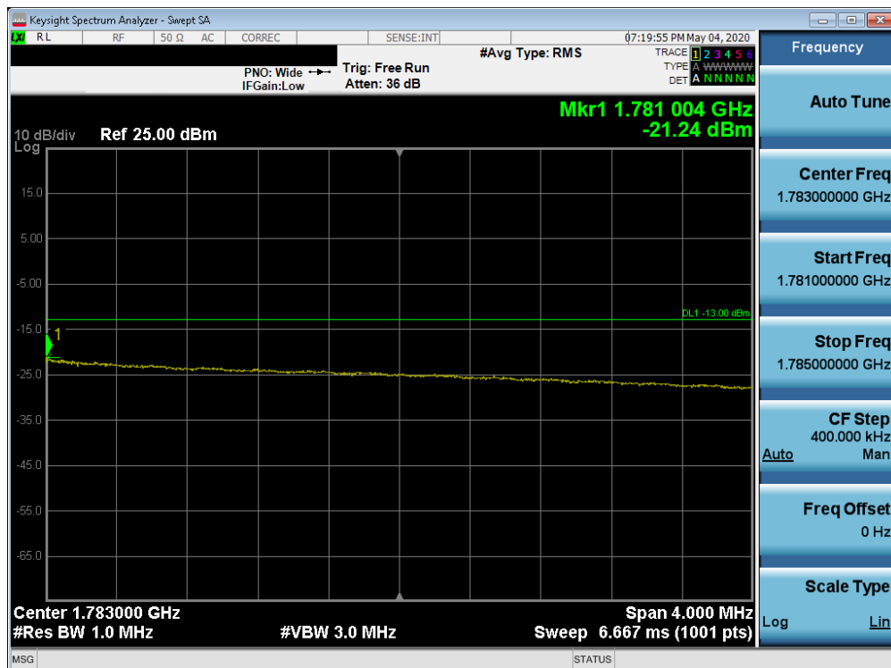
Plot 7-183. Upper Extended Band Edge Plot (Band 66 - 20.0MHz QPSK - Full RB Configuration)
