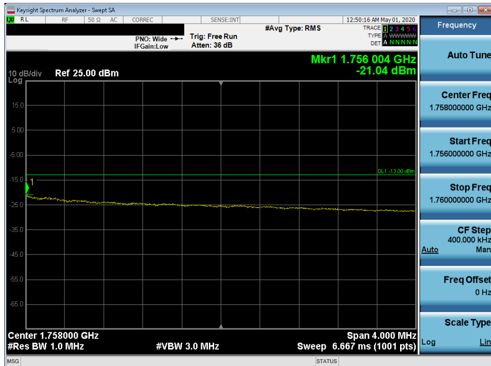
Plot 7-203. Upper Extended Band Edge Plot (Band 4 - 15.0MHz QPSK - Full RB Configuration)
