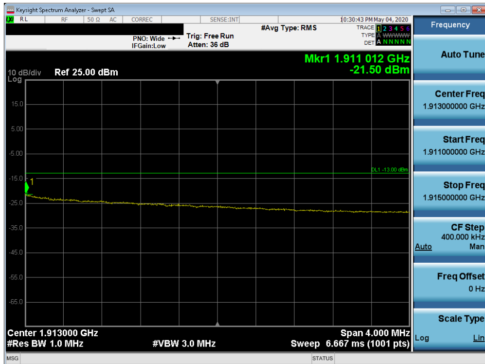
Plot 7-247. Upper Extended Band Edge Plot (Band 2 - 10.0MHz QPSK - Full RB Configuration)
