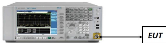
Figure 7-3. Test Instrument & Measurement Setup
