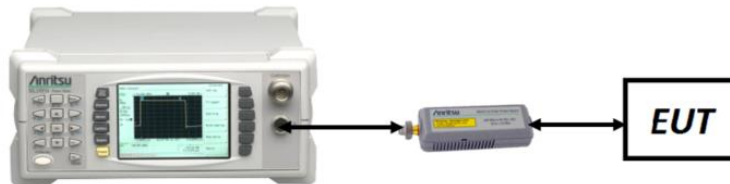
Figure 7-2. Test Instrument & Measurement Setup for Peak and Average Power Measurement
