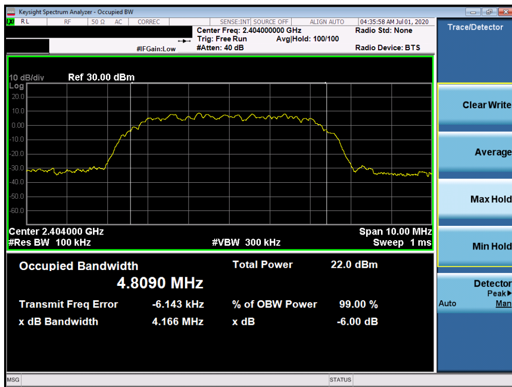
Plot 7-4. 6dB Bandwidth Plot (Bluetooth (HDR8), 8Mbps, ePA – Ch. 1)
