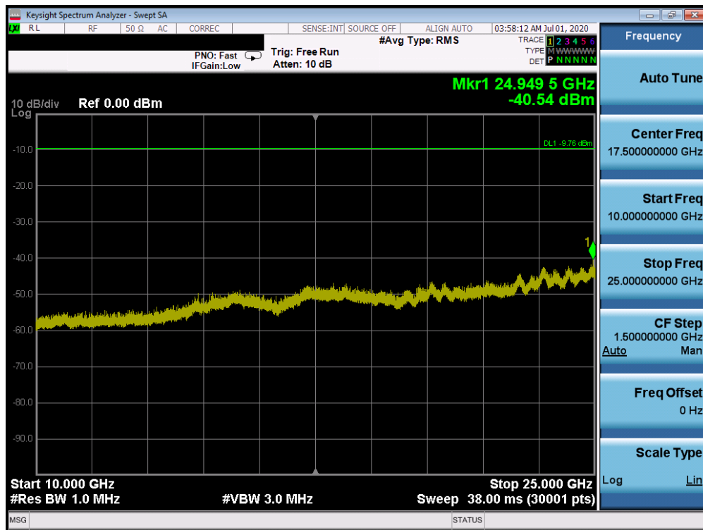
Plot 7-28. Conducted Spurious Plot (Bluetooth (HDR4), 4 Mbps, ePA – Ch. 75)
