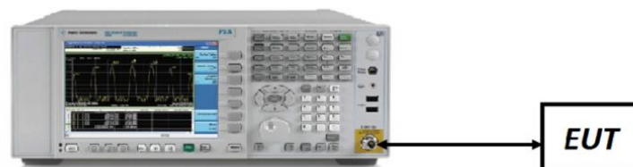
Figure 7-3. Test Instrument & Measurement Setup
