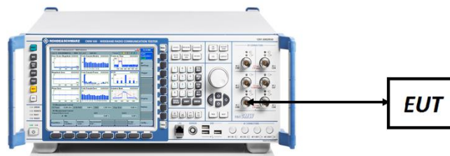
Figure 7-4. Conducted Power Measurement Setup
