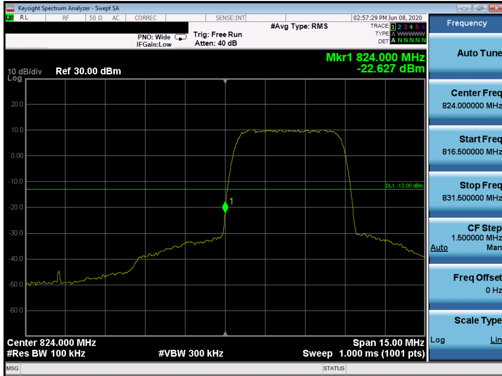
Plot 7-31. Band Edge Plot (Cellular WCDMA Mode - Low Channel)
