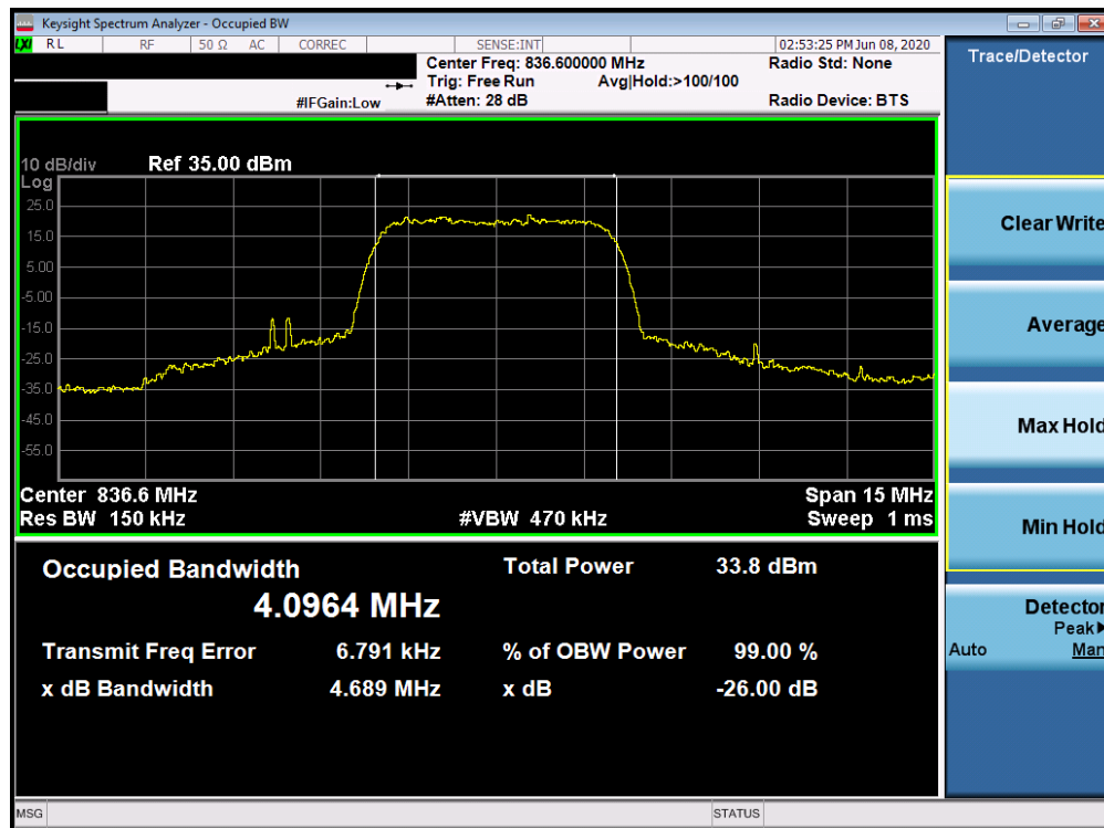
Plot 7-1. Occupied Bandwidth Plot (Cellular WCDMA Mode)
