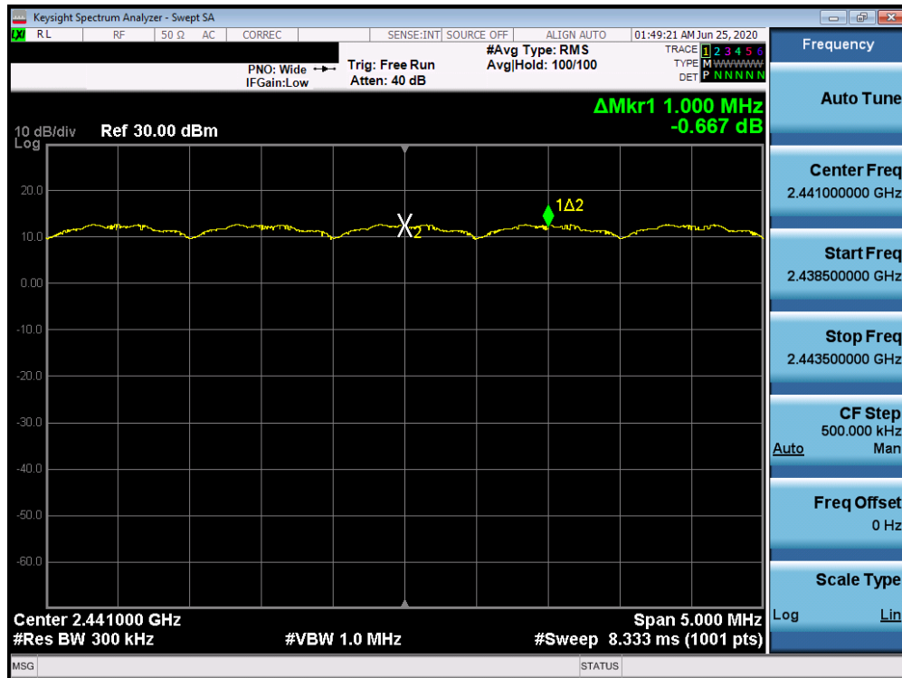
Plot 7-16. Channel Separation Plot (Bluetooth, 8DPSK, ePA)
