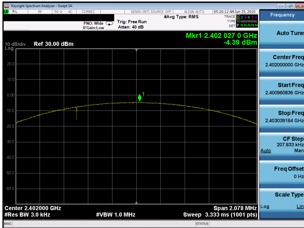
Plot 7-13. Power Spectral Density Plot (Bluetooth (LE), 2Mbps, ePA – Ch. 0)
