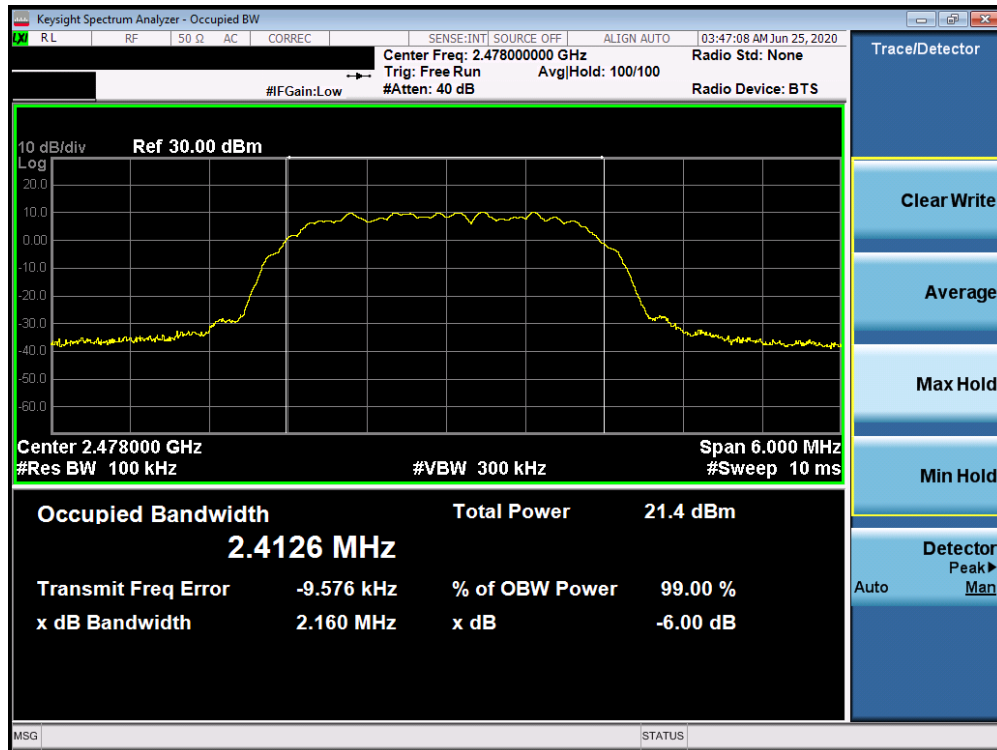
Plot 7-3. 6dB Bandwidth Plot (Bluetooth (HDR4), 4Mbps, ePA – Ch. 75)
