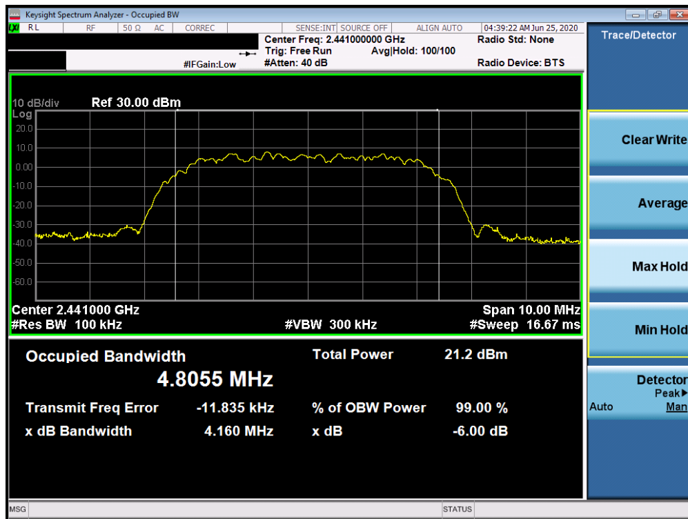
Plot 7-5. 6dB Bandwidth Plot (Bluetooth (HDR8), 8Mbps, ePA – Ch. 38)
