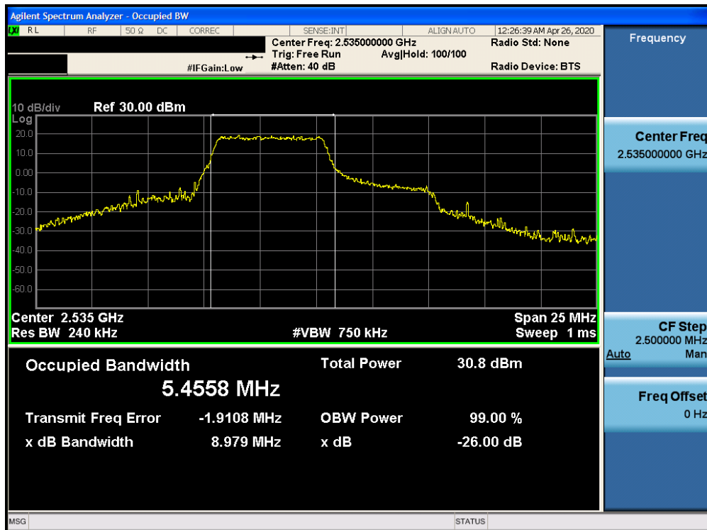
Plot 7-48. Occupied Bandwidth Plot (Band 7 - 10.0MHz 16-QAM - Full RB Configuration)
