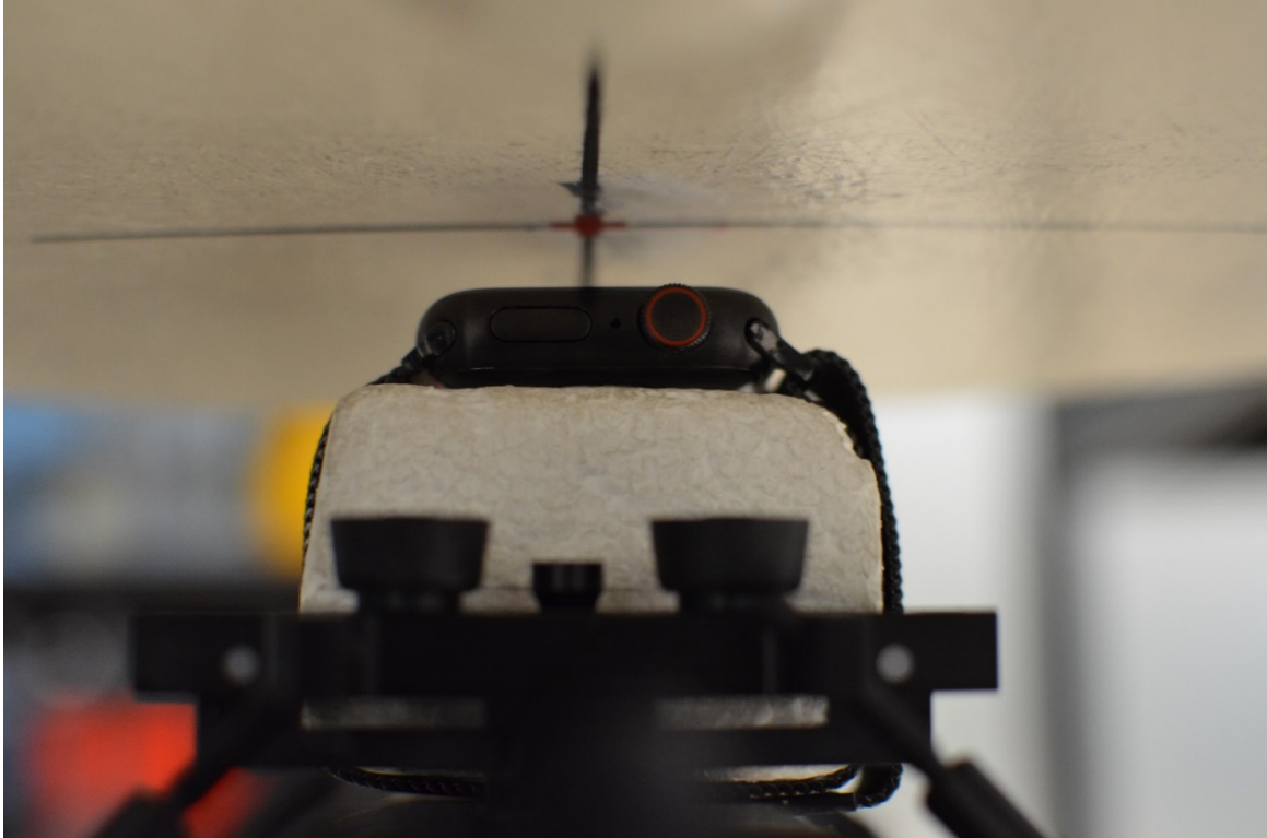
SAR Test Setup Photo 3: Aluminum with Metal Loop Wristband, Front side at 1.0 cm
