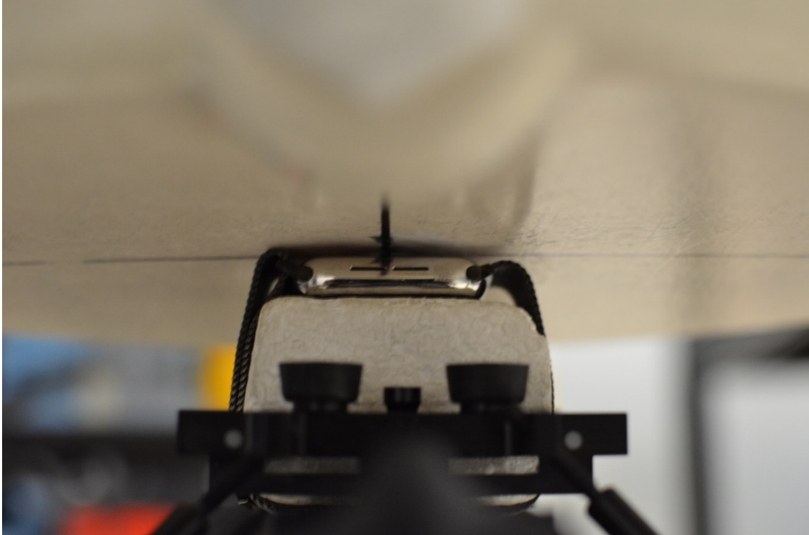
SAR Test Setup Photo 15: Stainless Steel with Metal Loop Wristband, Back side at 0.0 cm
