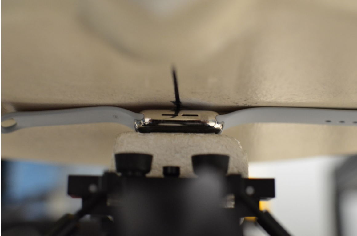
SAR Test Setup Photo 13: Stainless Steel with Sport Wristband, Back side at 0.0 cm
