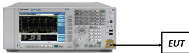
Figure 7-1. Test Instrument & Measurement Setup
