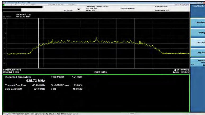
Plot 7-28. ISED Occupied Bandwidth (Ch. 5, Config 3/Payload 125)
