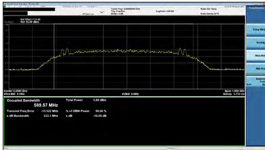
Plot 7-31. ISSED Occupied Bandwidth (Ch. 9, Config 0/Payload 25)
