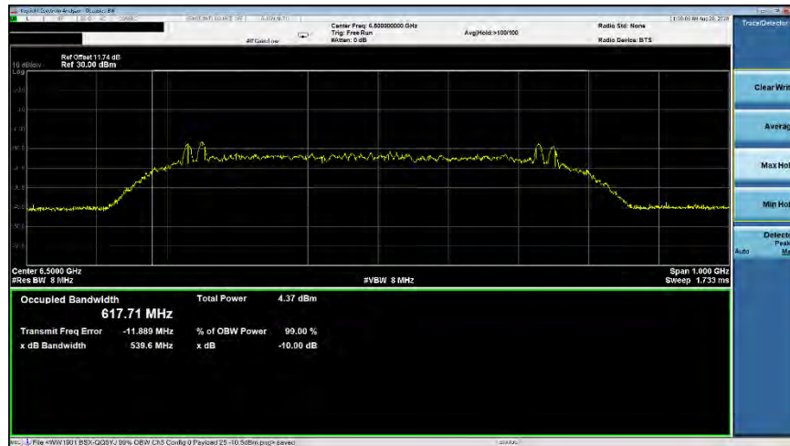
Plot 7-22. ISSED Occupied Bandwidth (Ch. 5, Config 0/Payload 65)
