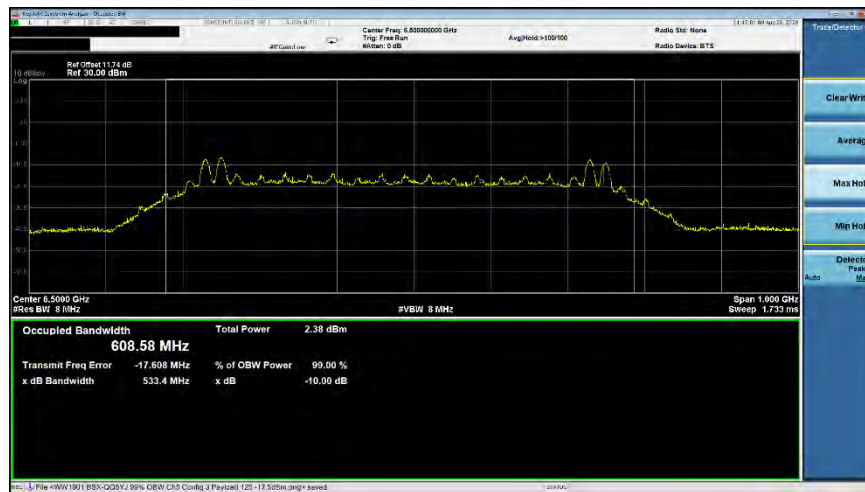
Plot 7-29. ISED Occupied Bandwidth (Ch. 5, Config 4/Payload 0)
