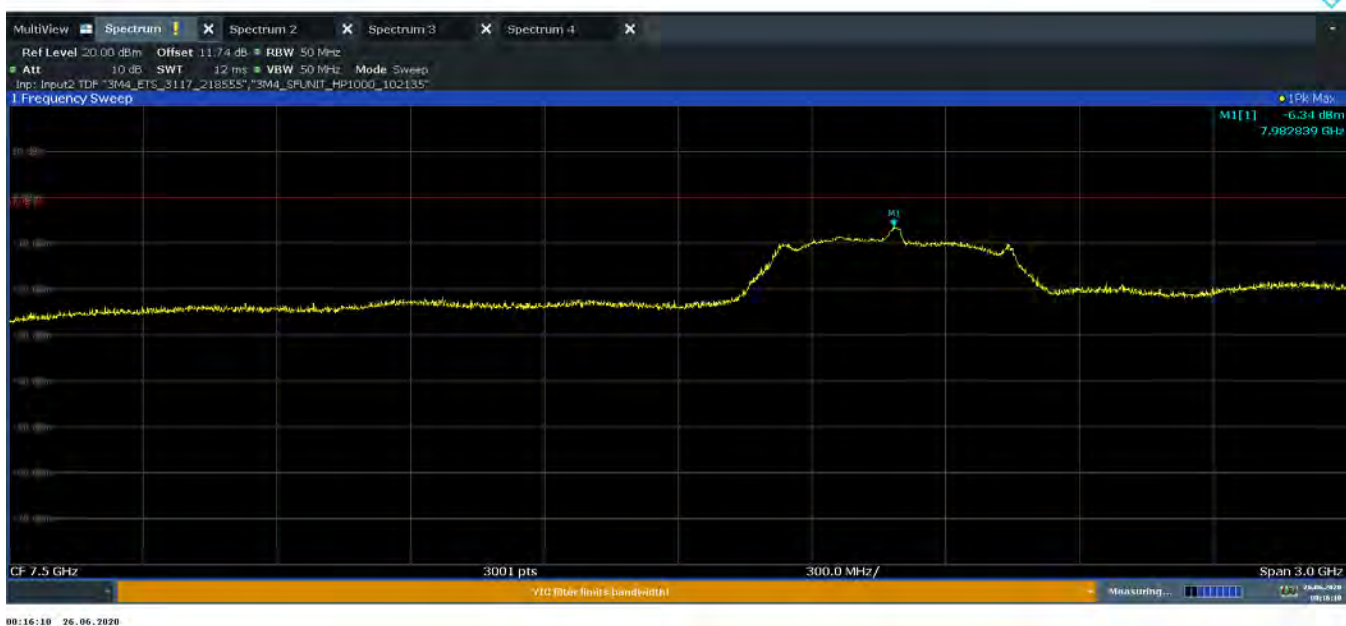
Plot 7-58. Peak Radiated Power (Ch. 9, Config 3/Payload 125)
