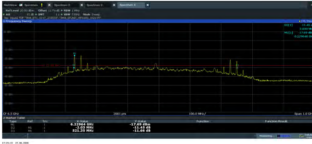
Plot 7-7. 10dBc Bandwidth (Ch. 5, Config 2/Payload 125)
