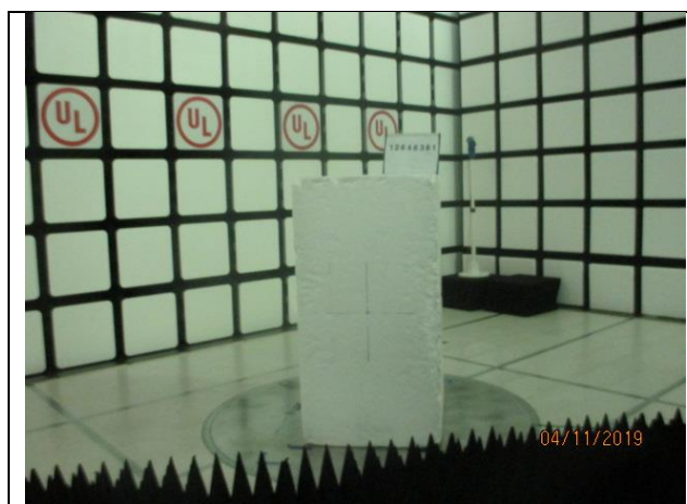
ABOVE 1GHz X-Axis Front
