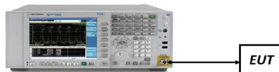
Figure 7-5. Test Instrument & Measurement Setup
