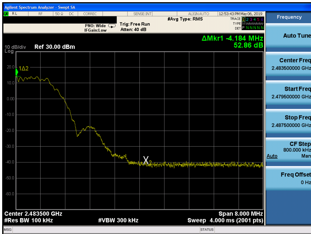
Plot 7-22. Band Edge Plot (Bluetooth (LE), 2Mbps ePA – Ch. 39)
