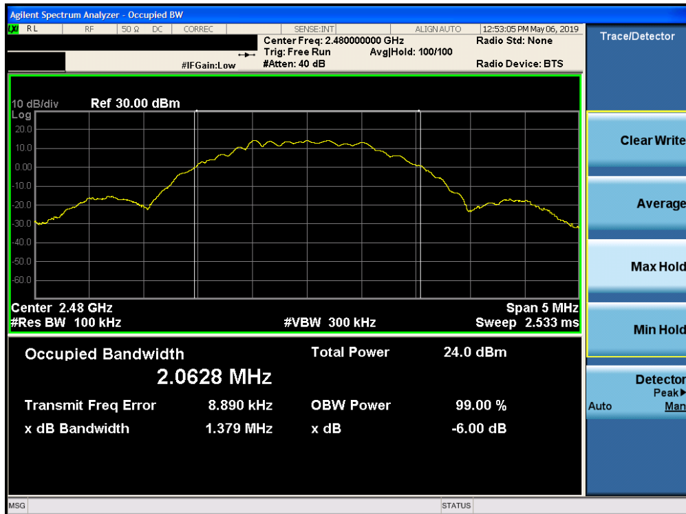
Plot 7-6. 6dB Bandwidth Plot (Bluetooth (LE), 2Mbps ePA – Ch. 39)
