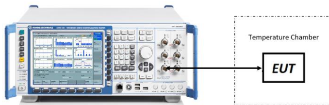
Figure 7-7. Test Instrument & Measurement Setup
