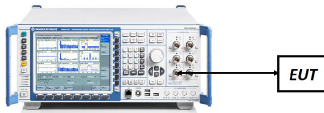
Figure 7-4. Conducted Power Measurement Setup
