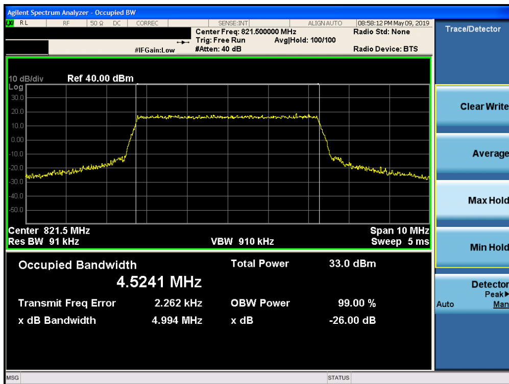
Plot 7-5. Occupied Bandwidth Plot (LTE Band 26, 5MHz QPSK – RB Size 25– High Channel)
