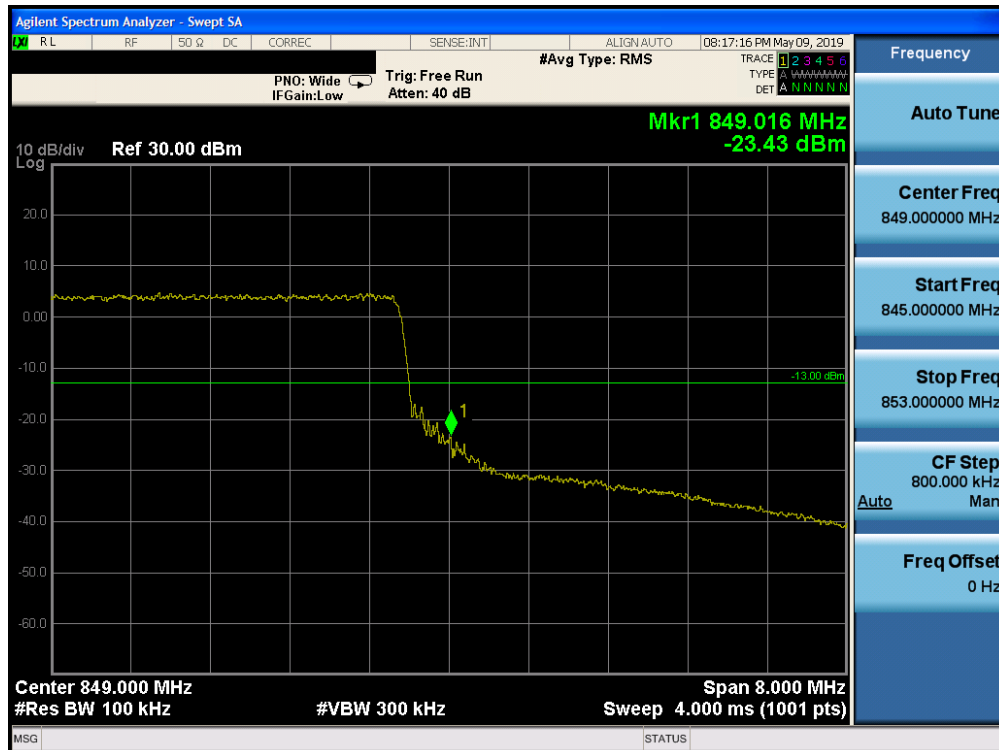
Plot 7-101. Upper Band Edge Plot (Band 26 - 10.0MHz QPSK - Full RB Configuration)
