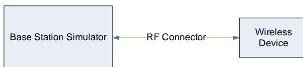
Figure 8-1 Power Measurement Setup
