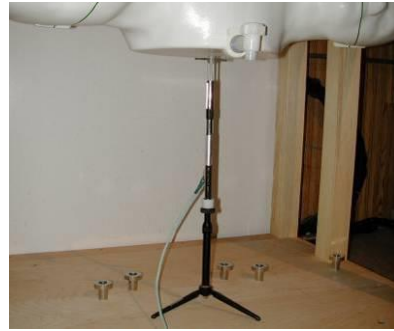
Figure 9-2 System Verification Setup Photo
