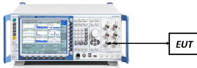
Figure 7-4. Conducted Power Measurement Setup
