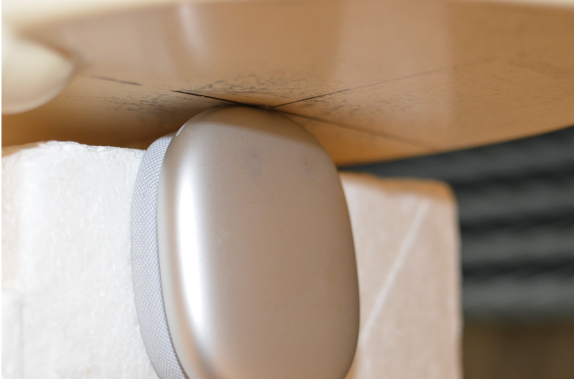
SAR Test Setup Photo 3: Bottom Edge Extremity SAR at 0.0 cm
