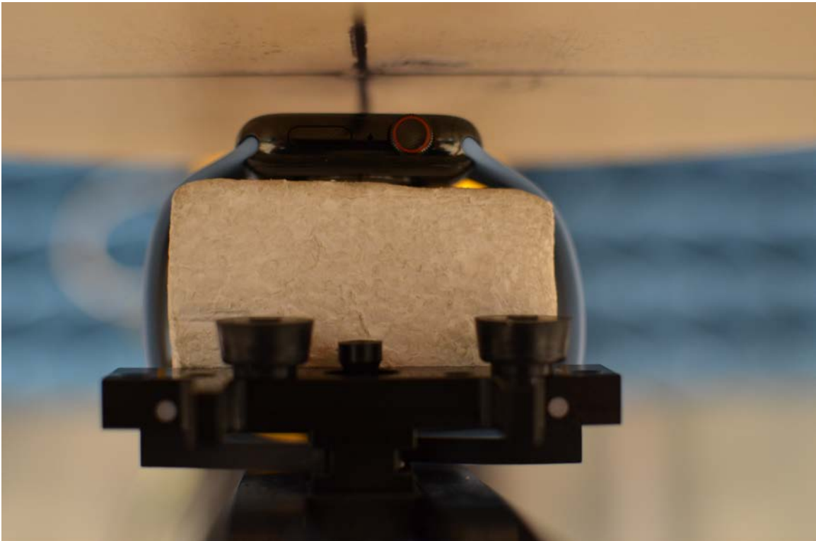
SAR Test Setup Photo 4: Stainless Steel with Sport Wristband, Front side at 1.0 cm
