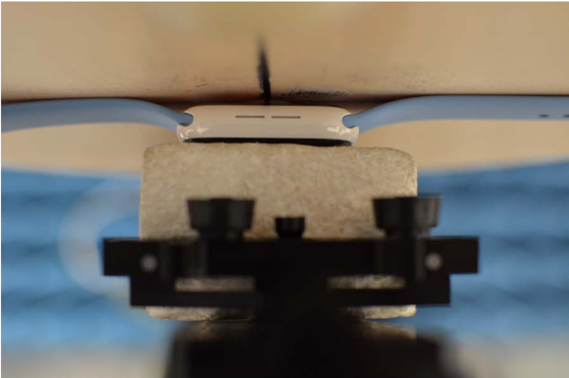
SAR Test Setup Photo 22: Ceramic with Sport Wristband, Back side at 0.0 cm
