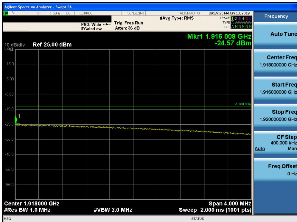
Plot 7-227. Upper Extended Band Edge Plot (Band 25 - 20.0MHz QPSK - Full RB Configuration)
