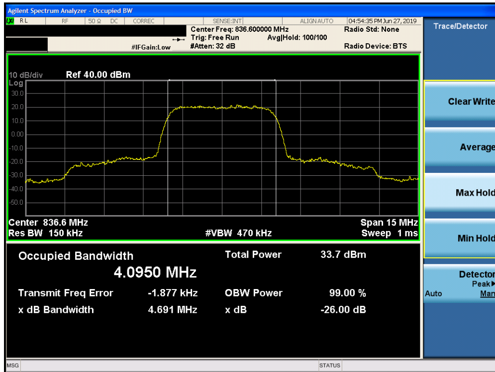
Plot 7-1. Occupied Bandwidth Plot (Cellular WCDMA Mode)
