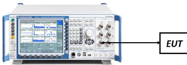
Figure 7-5. ERP/EIRP Measurement Setup
