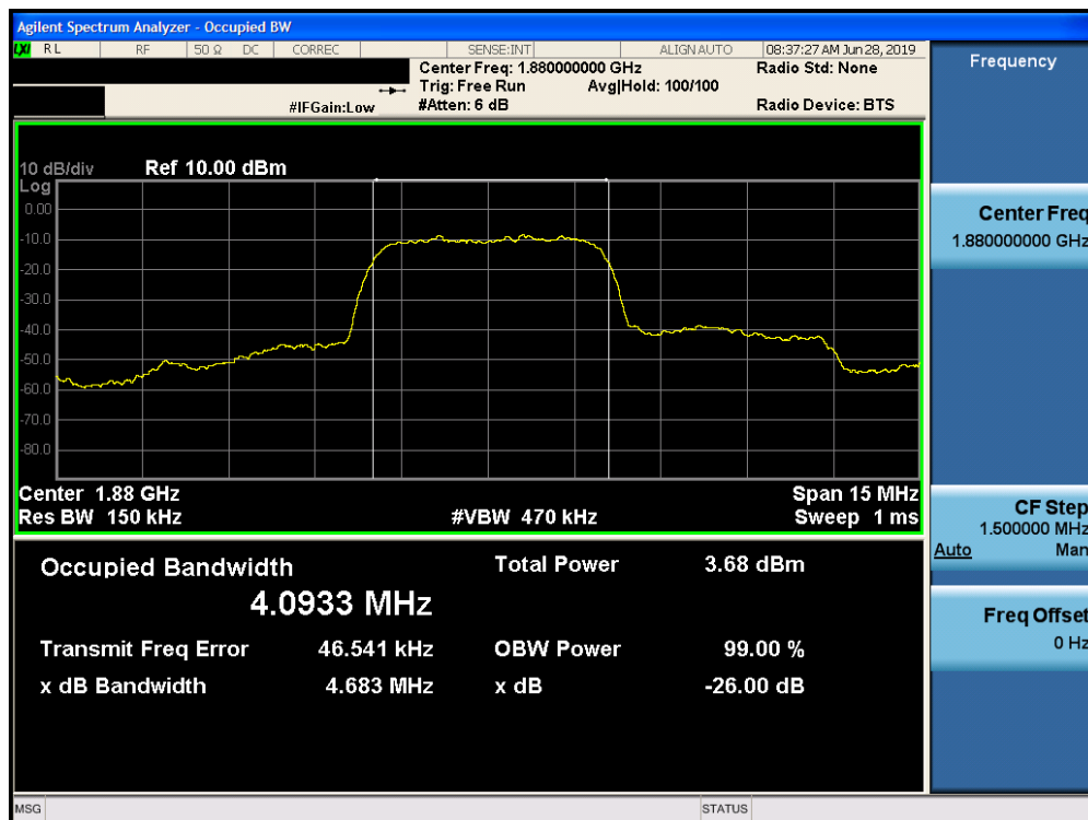
Plot 7-3. Occupied Bandwidth Plot (PCS WCDMA Mode)
