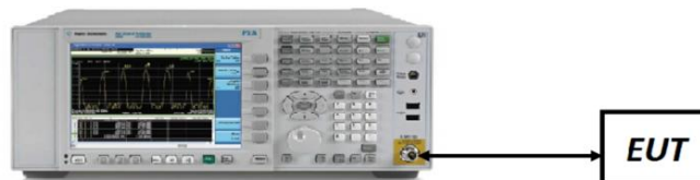
Figure 7-3. Test Instrument & Measurement Setup
