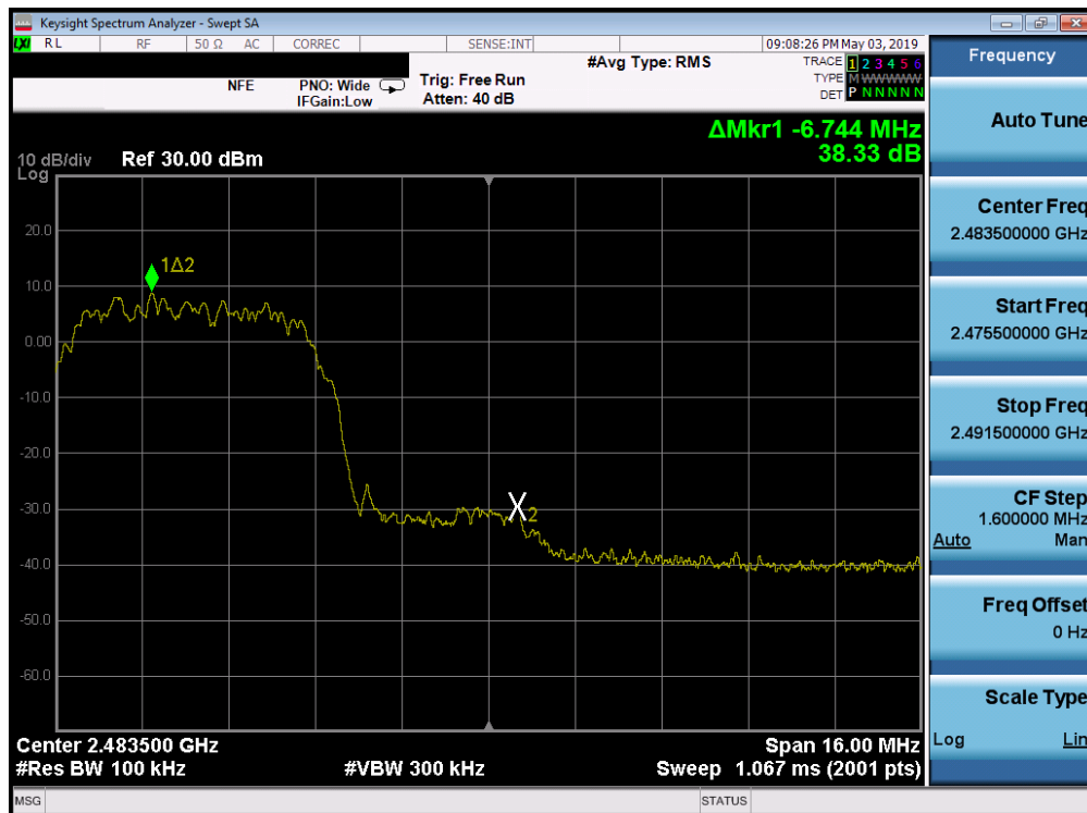
Plot 7-22. Band Edge Plot (Bluetooth (HDR8), ePA – Ch. 75)
