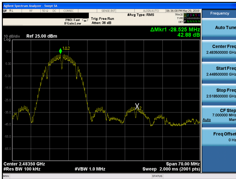
Plot 7-21. Band Edge Plot (802.11b – Ch. 12)
