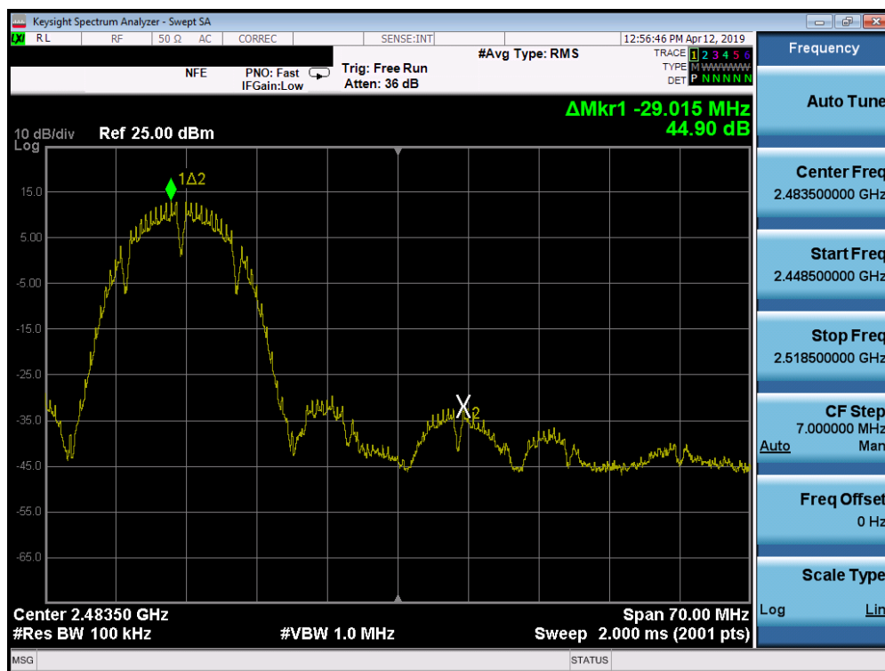
Plot 7-20. Band Edge Plot (802.11b – Ch. 11)
