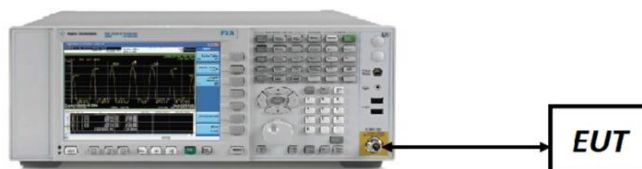
Figure 7-3. Test Instrument & Measurement Setup
