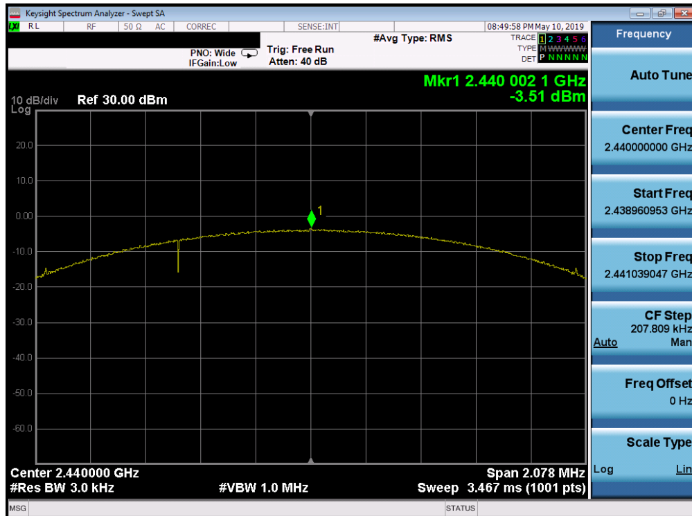
Plot 7-14. Power Spectral Density Plot (Bluetooth (LE), 2Mbps ePA – Ch. 19)
