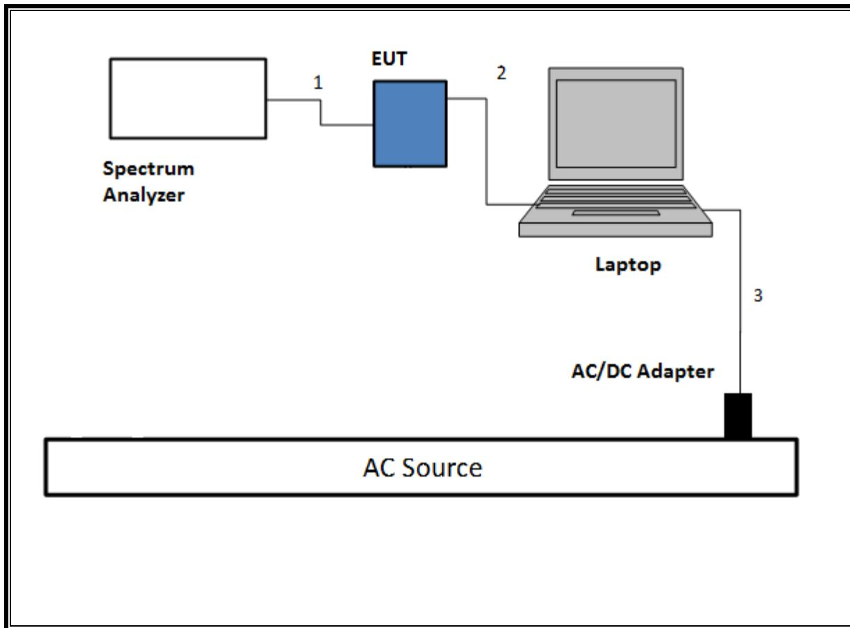
**SETUP DIAGRAM FOR RADIATED TESTS ABOVE 1GHz**
