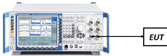
Figure 7-4. Conducted Power Measurement Setup
