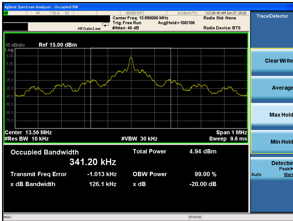
Figure 7-5. 20dB Bandwidth Plot (Reader 100% Ask 1 out of 4)
