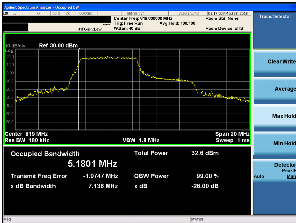
Plot 7-8. Occupied Bandwidth Plot (10MHz 16-QAM – RB Size 27, RB Offset 0 Configuration)
