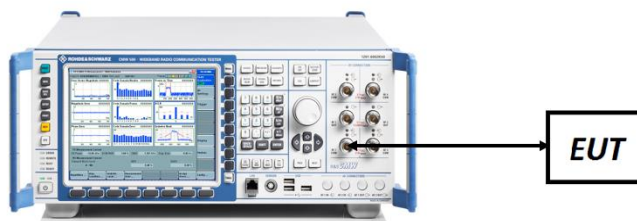
Figure 7-4. ERP/EIRP Measurement Setup
