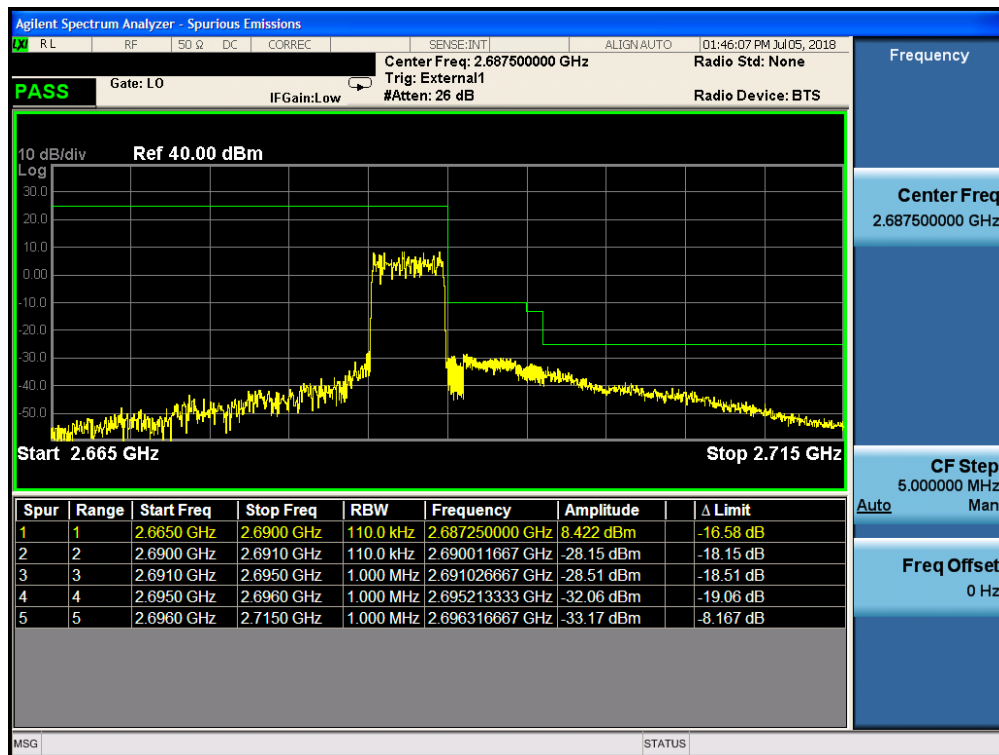
Plot 7-78. Upper ACP Plot (Band 41 - 5.0MHz QPSK - RB Size 25)
